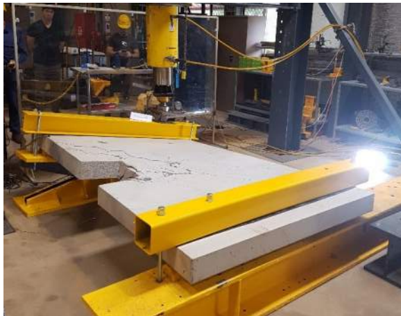
Testing of GFRP-reinforced precast planks under torsion
