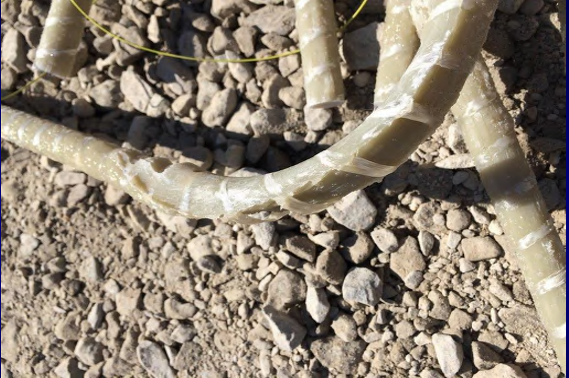
Unacceptable bar with loose helical wrap, voids and kinks in fibre
