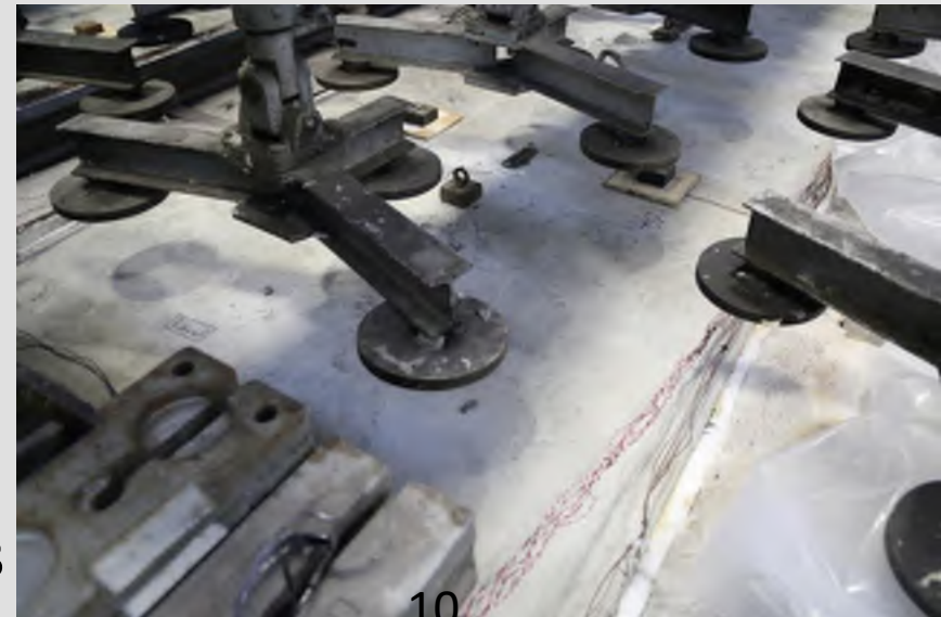
Uniform loading on the slabs
