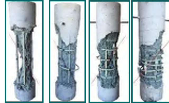
Increasing degree of concrete crushing failure
