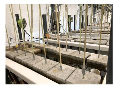
Figure 3: Exposure process of bond samples
