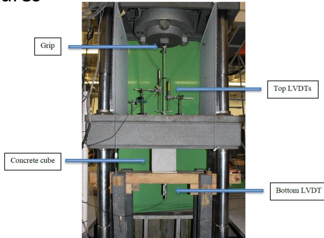
Figure 4: 'Pull-out test' configuration per ASTM D793
