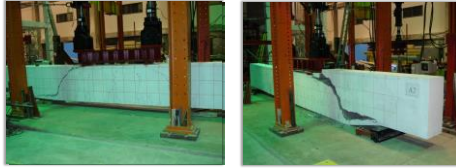
Beam B1-1 Beam B1-2 Diagonal Tension Failure Mode
