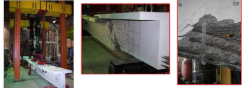
Shear Failure of SC-9.5-2 (CFRP @ d/2)
