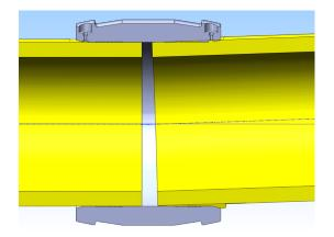
Mis-Alignment- Unacceptable Fusion Possible Causes: Inadequate Clamping or Restraint during fusion.
