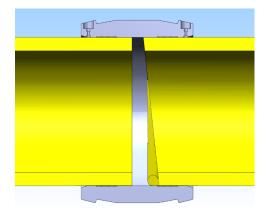
Mis-Cut- Unacceptable Fusion Possible Causes: Failure to cut the pipe end perpendicular to the axis of the pipe.
