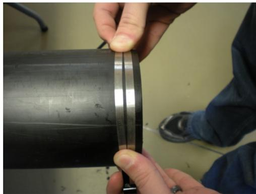
Measure pipe with a pipe diameter tape
