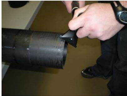
Deburring or Beveling pipe ends
