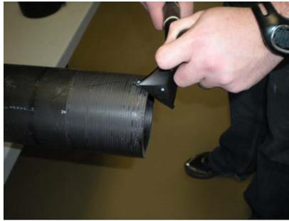
Deburring or Beveling pipe ends
