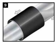
Slide the tube onto the steel joint area, positioning the weld seam at the 12 o'clock position (if applicable). Centre the tube to ensure a minimum 50 mm (2") overlap onto the pipe coating. Remove the protective paper lining prior to shrinkdown.
