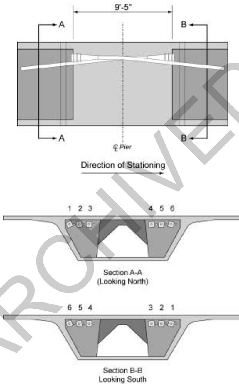
Figure 1.6 – Tendon Numbering Convention (Interior Piers)
