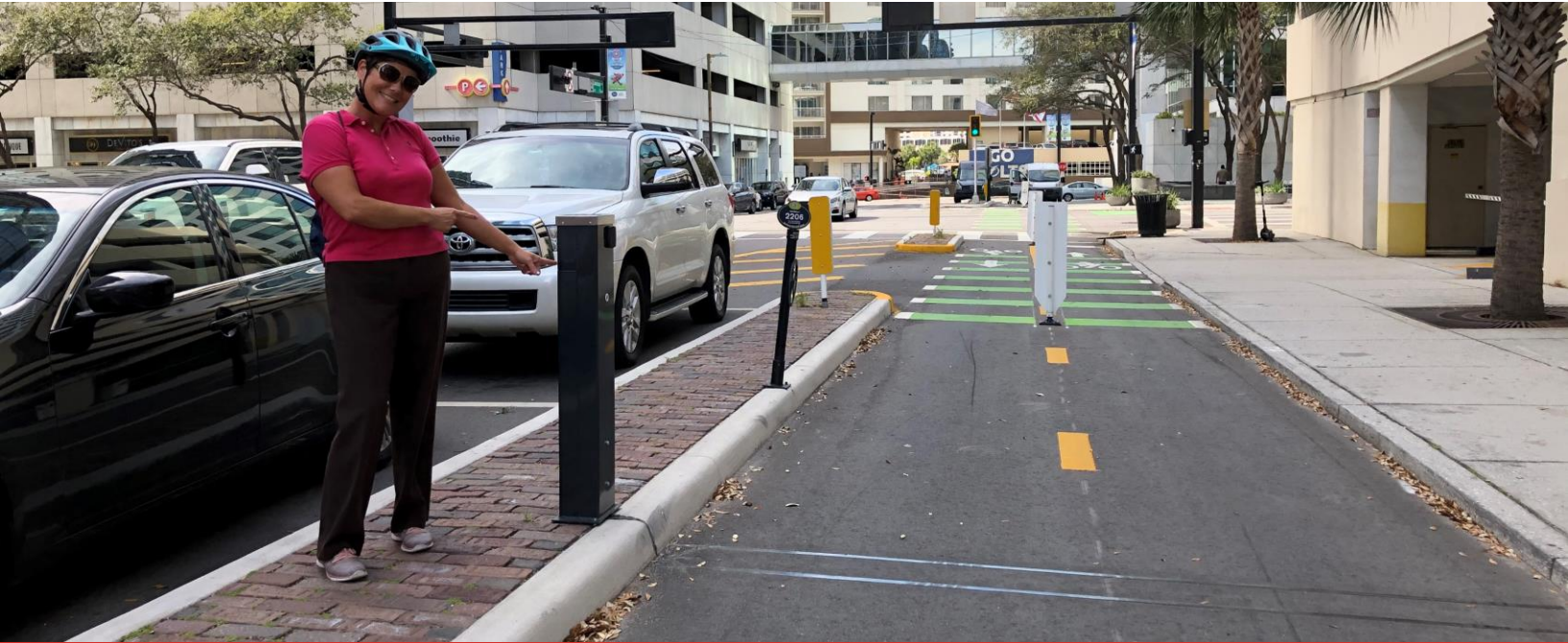
Recent continuous counter installation along Jackson St. Cycle track in downtown Tampa (Photo courtesy Stephanie Moss)
