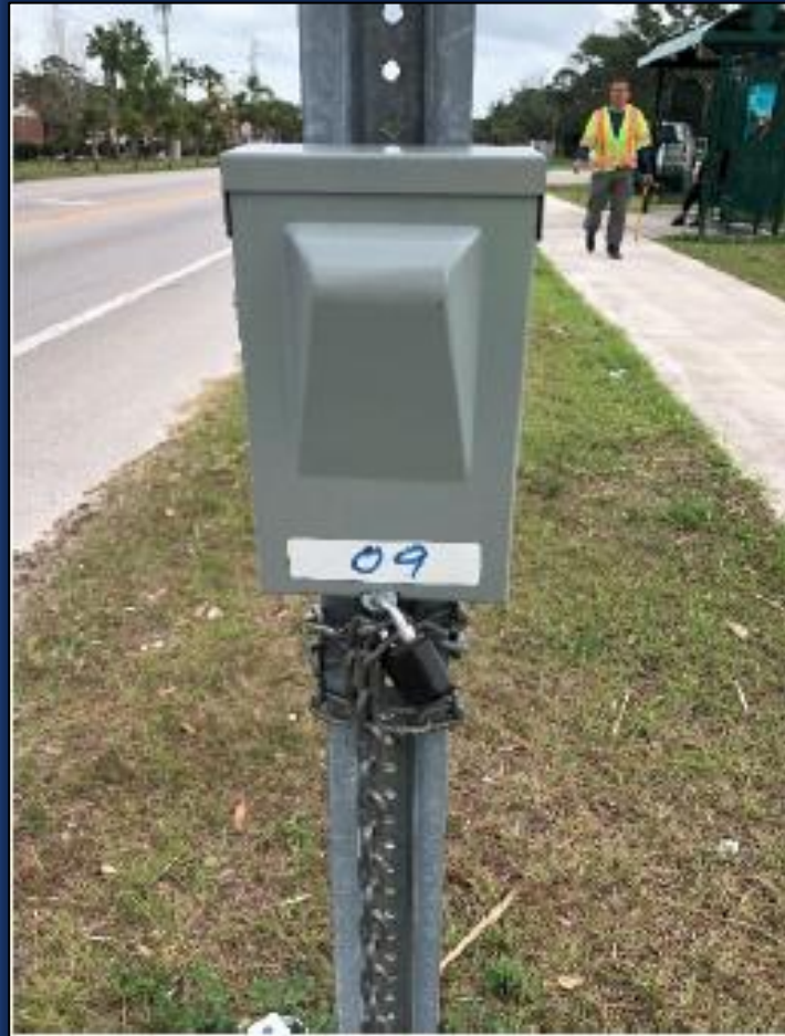
INFRARED DEVICE USED TO COUNT ACTIVITY ON SIDEWALK
