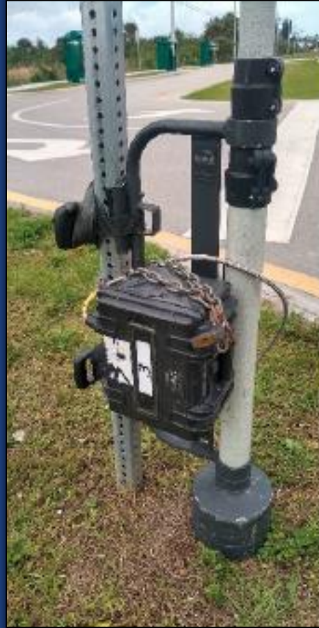
VIDEO CAMERA ON TELESCOPING POLE TO RECORD ALL ACTIVITY
