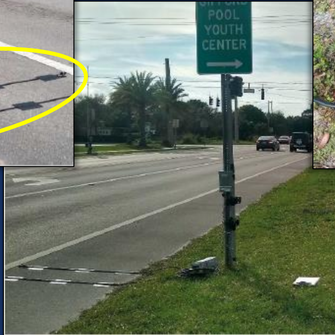
BIKE TUBE COUNTERS USED TO COUNT BICYCLE ACTIVITY IN BICYCLE LANES AND ON BIKE PATHS
