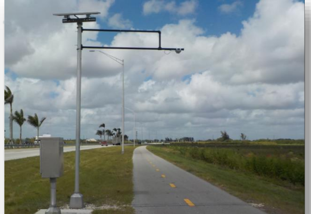
Krome Path, West Kendall, Miami-Dade County Overhead Infrared with piezo-electric sensors 2023 Avg. Daily Users: 58
