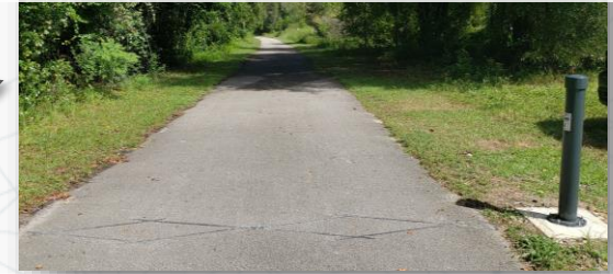
Withlacoochee State Trail, Floral City, Citrus County Side Fire Infrared with Inductive Loops 2023 Avg. Daily Users: 257
