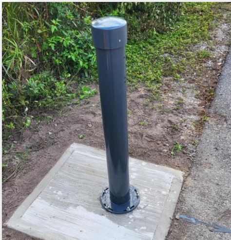
Legacy Trail, Sarasota, Sarasota County Side Fire Infrared with Inductive Loops 2023 Avg. Daily Users: 755
