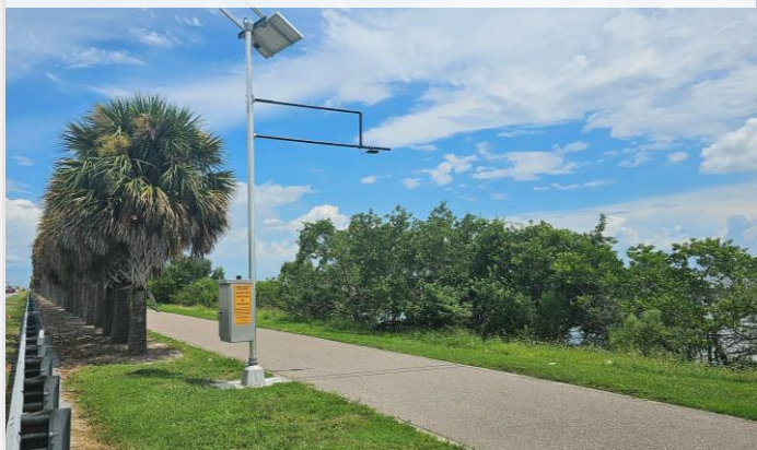
Courtney Campbell Causeway, Clearwater, Pinellas County Overhead Infrared with piezo-electric sensors 2023 Avg. Daily Users: 414
