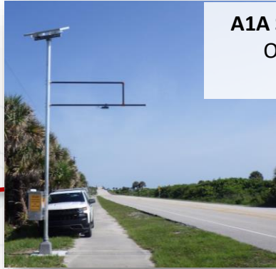
Trans FL Rail Trail, Fellsmere, Indian River County Overhead Infrared with piezo-electric sensors 2023 Avg. Daily Users: 54
