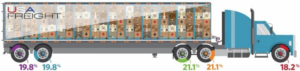
Figure 3 - Full Class 9 Truck Axle Weight Load Distribution
