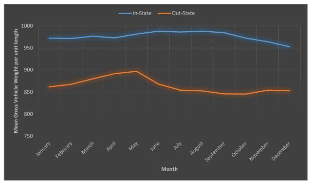
Figure 12 - Monthly Mean Gross Vehicle Weight Per Unit Length of Truckload (lbs/ft)
