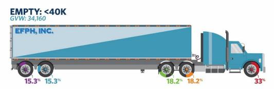
Figure 4 - Empty Class 9 Truck Axle Weight Load Distribution
