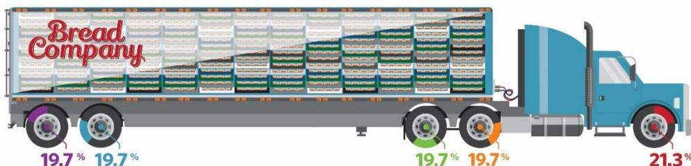
Figure 5 - Full Volume but Light Weight Class 9 Truck Axle Weight Load Distribution
