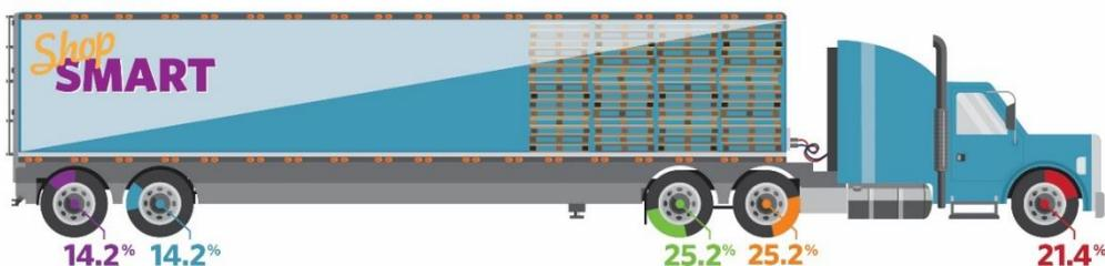
Figure 6 - Partially Empty Class 9 Truck Axle Weight Load Distribution
