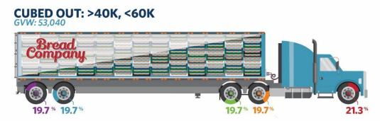
Figure 5 - Full Volume but Light Weight Class 9 Truck Axle Weight Load Distribution
