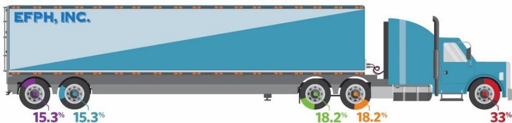
Figure 4 - Empty Class 9 Truck Axle Weight Load Distribution
