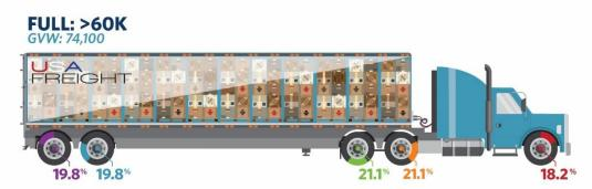
Figure 3 - Full Class 9 Truck Axle Weight Load Distribution
