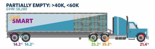
*Figure 6 - Partially Empty Class 9 Truck Axle Weight Load Distribution*
