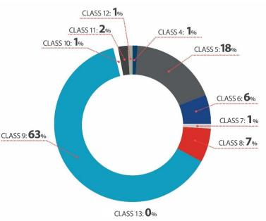
Figure 11 - Percentage of Trucks by different vehicle classes passing through the WIM sites on the Interstate system
