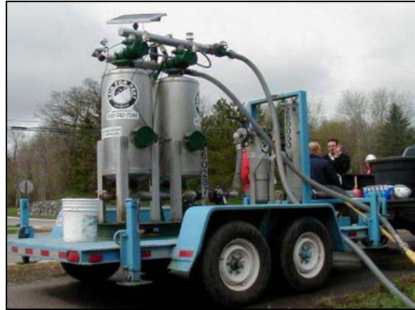
Sand Media Particulate Filter
