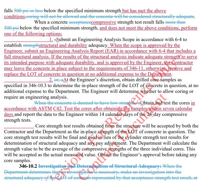
Department determines that an investigation is necessary, make an investigation into the structural adequacy of the LOT of concrete represented by that acceptance strength test result, at no additional expense to the Department. The Engineer may also require the Contractor to perform additional testing as necessary to determine structural adequacy of the concrete.
