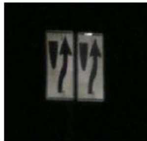
close up of sign faces viewed from sedan low beam VOA headlights
