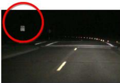
The same Keep Right signs viewed at night, sedan, low beam VOA headlights
