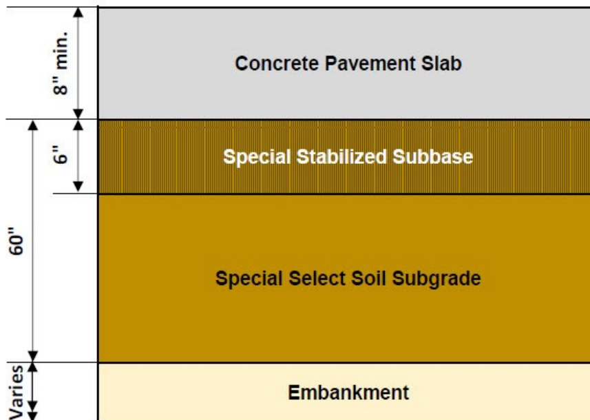
FIGURE 2.2 SPECIAL SELECT SOIL BASE OPTION
