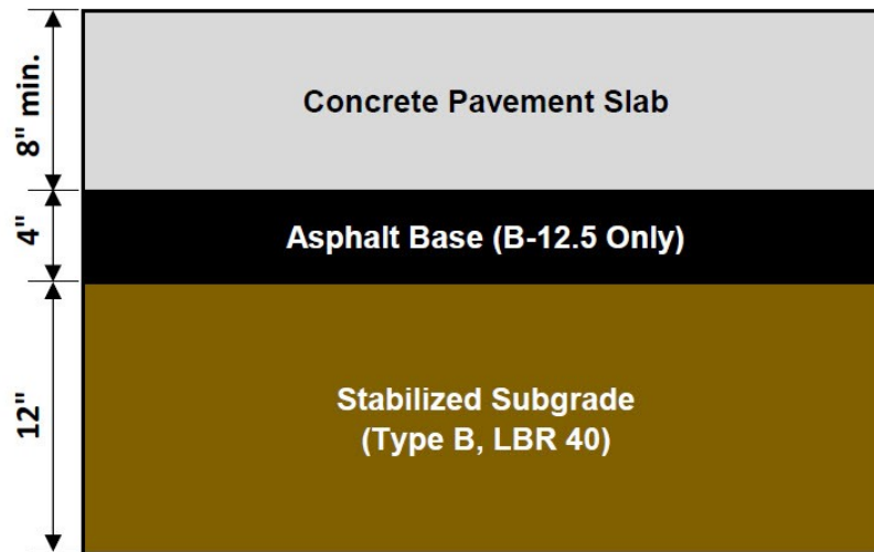
FIGURE 2.2 SPECIAL SELECT SOIL BASE OPTION
