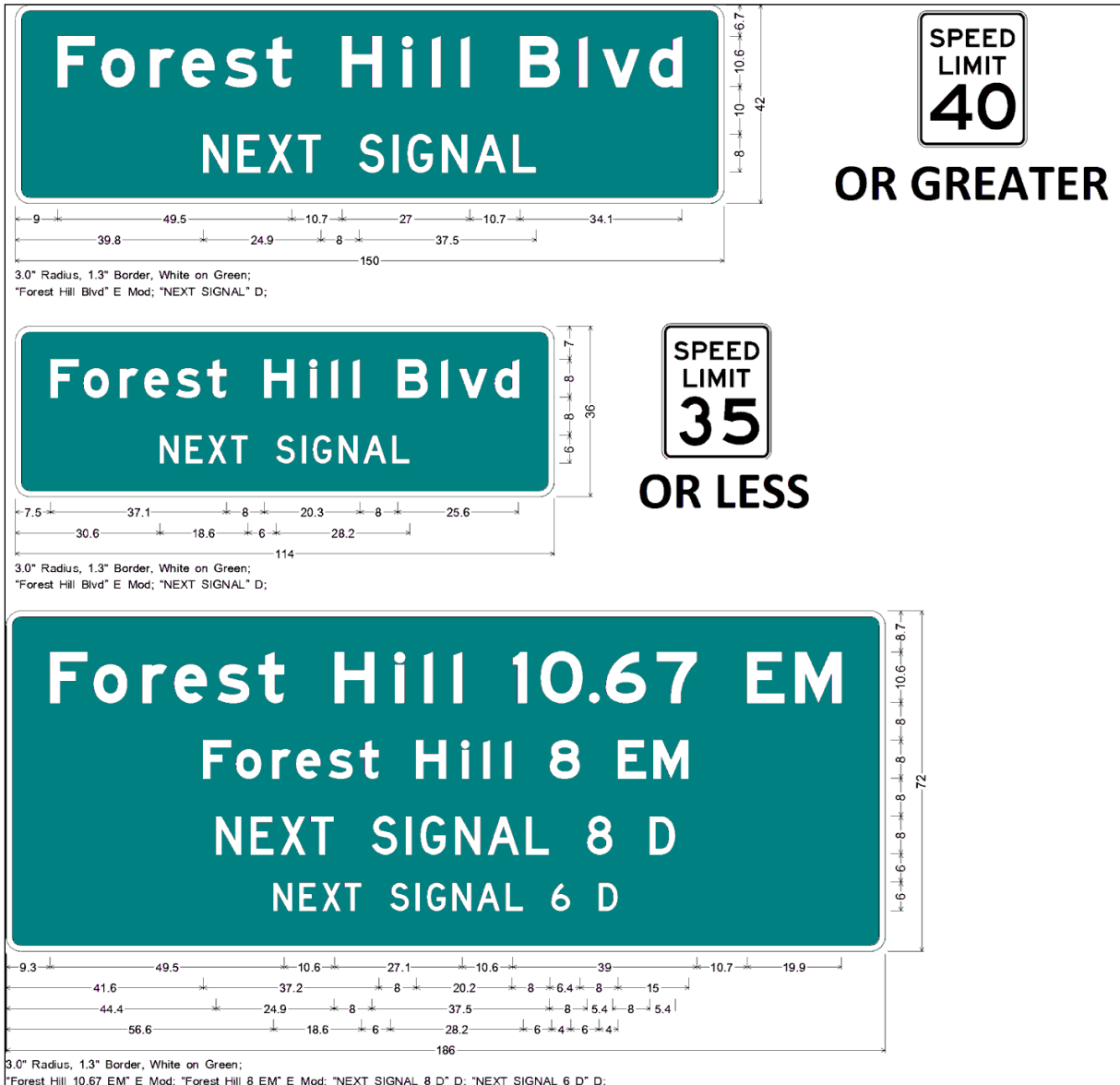
Figure 18 – 1 Examples of Advance Street Name Signs
