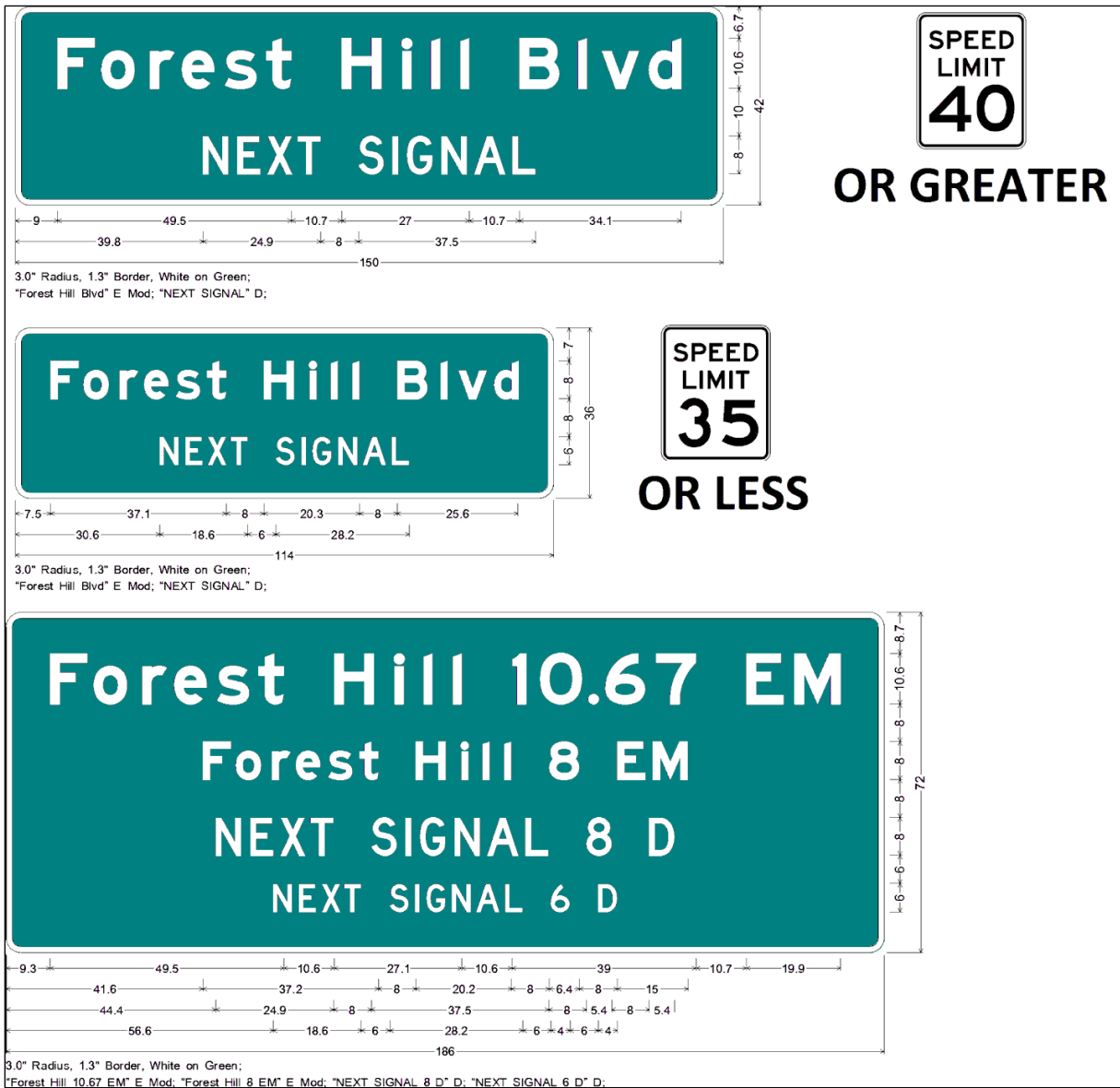
Figure 18 – 1 Examples of Advance Street Name Signs
