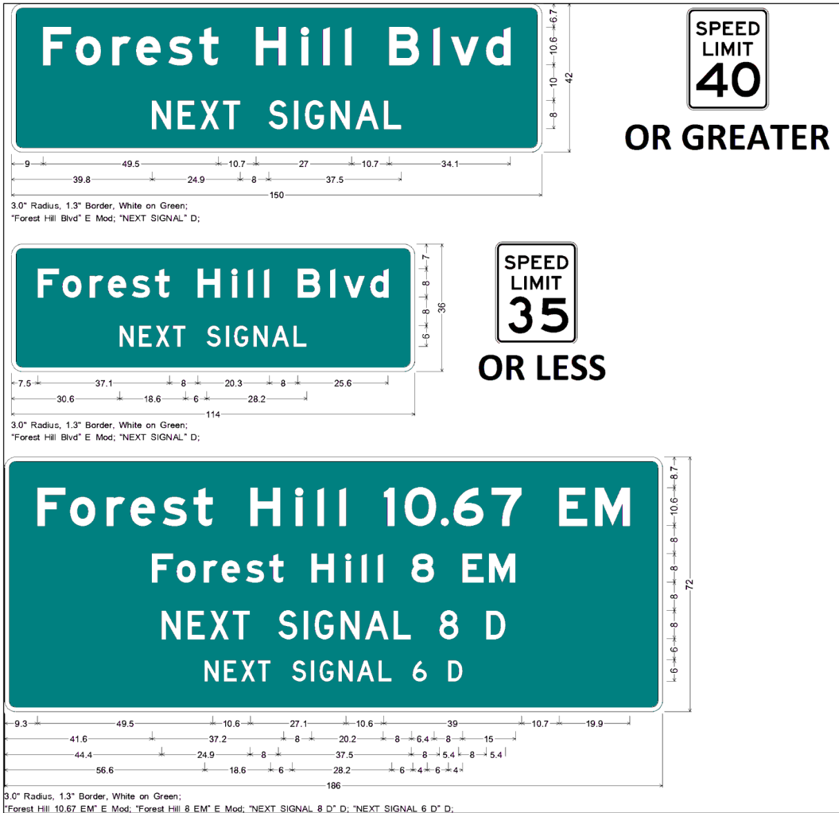
Figure 18 – 1 Examples of Advance Street Name Signs
