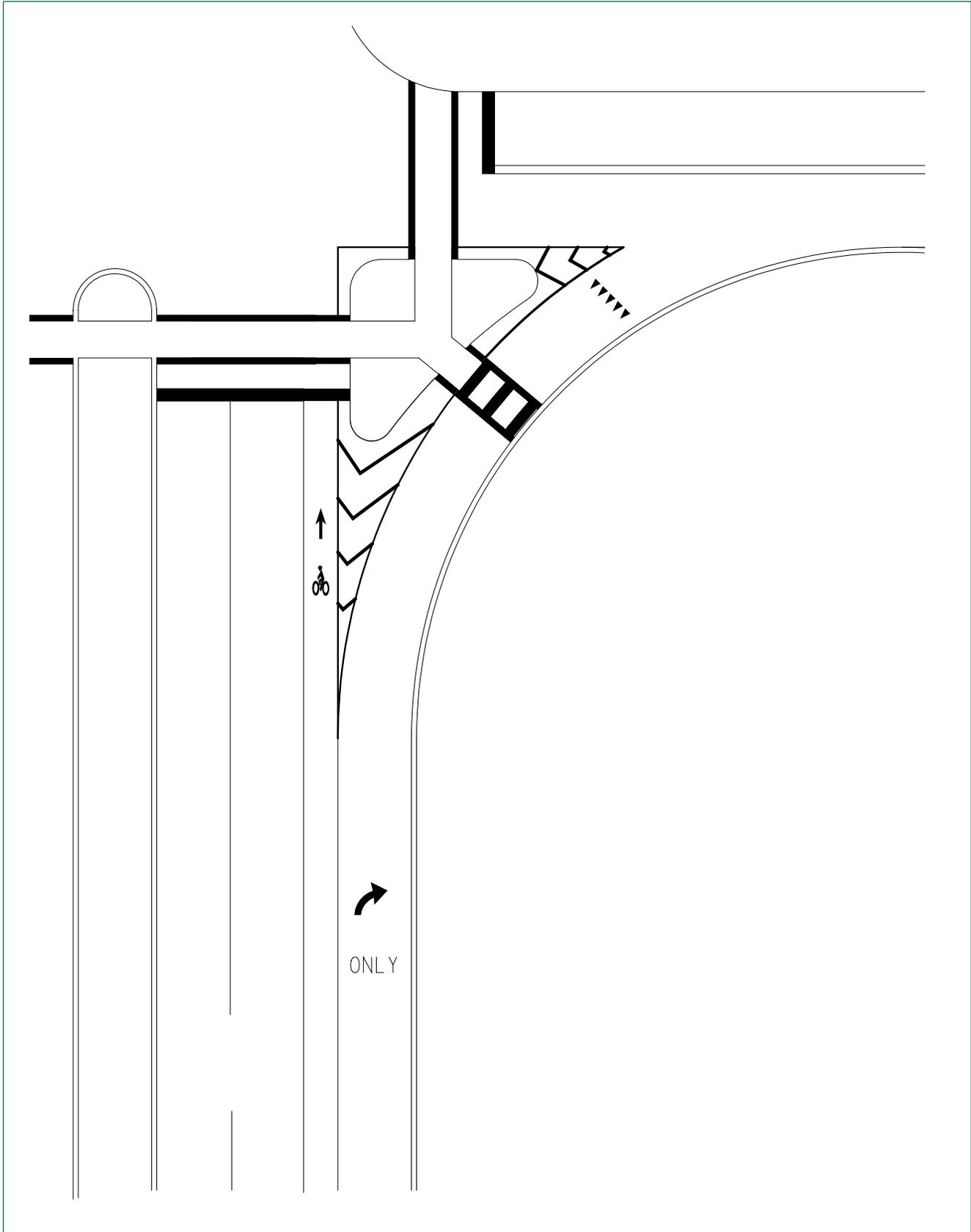
**Figure 3-8 Details of Corner Island for Turning Roadways (Curbed)**
