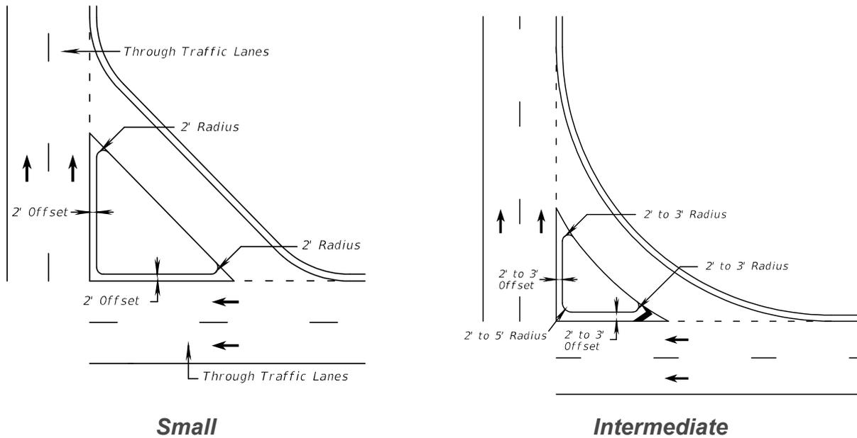
**Figure 3-9 Details of Corner Island for Turning Roadways (Flush Shoulder)**
