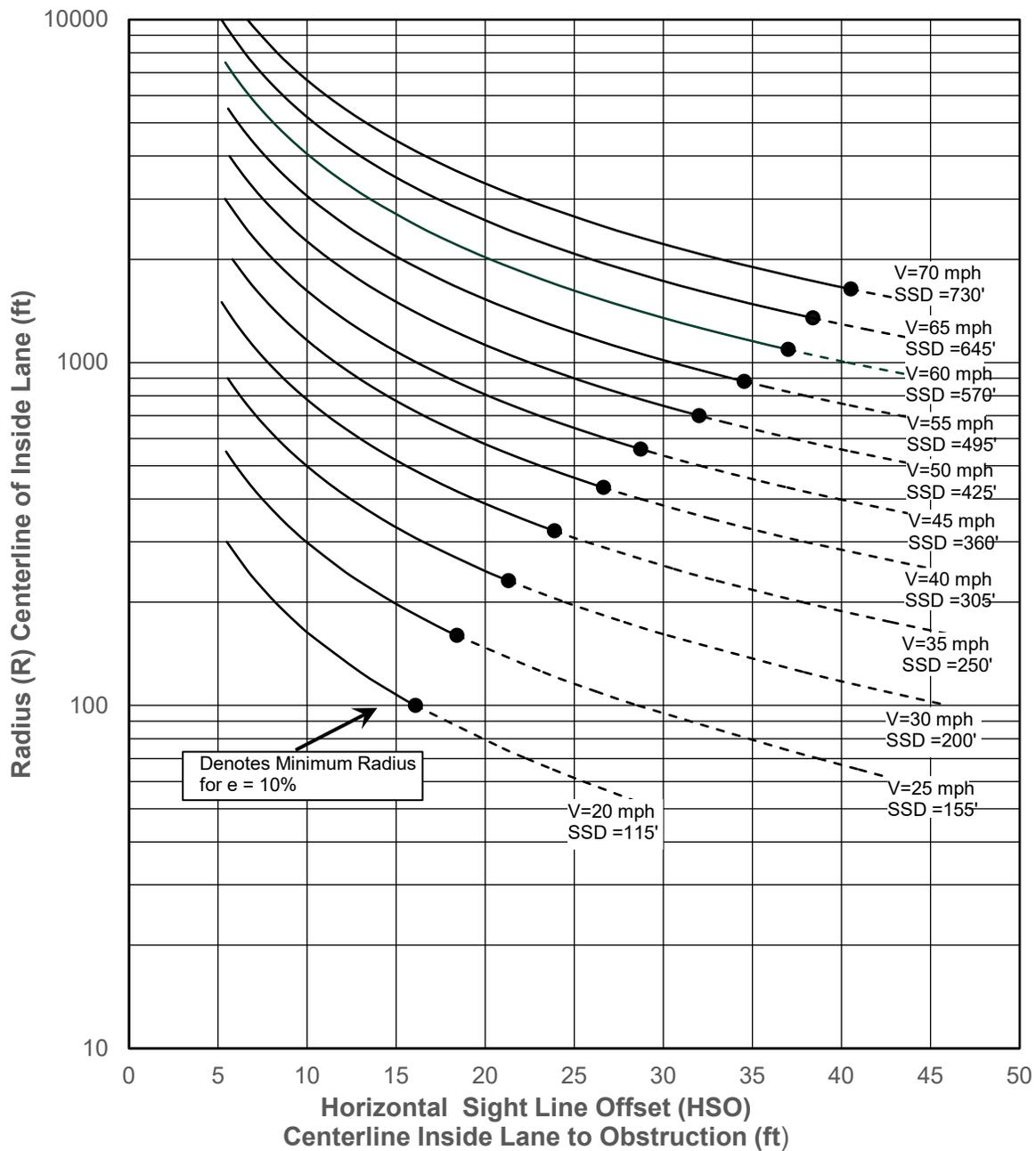
**Figure 3-2** Diagram Illustrating Components for Determining Horizontal Sight Distance
