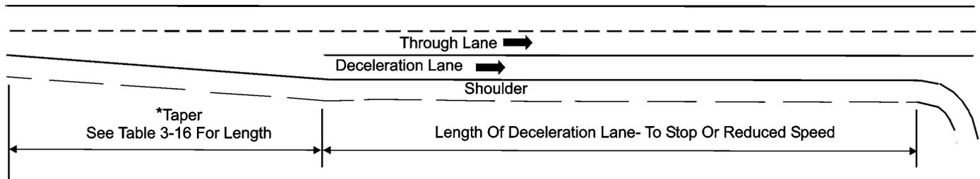
\*As An Alternate Acceptable Design, The Taper Can Be Set At A 50 Ft. Length With The Additional Length Of Normal Taper Added To The Deceleration Length. This Allows For Vehicles To Exit The Through Lane Earlier.
