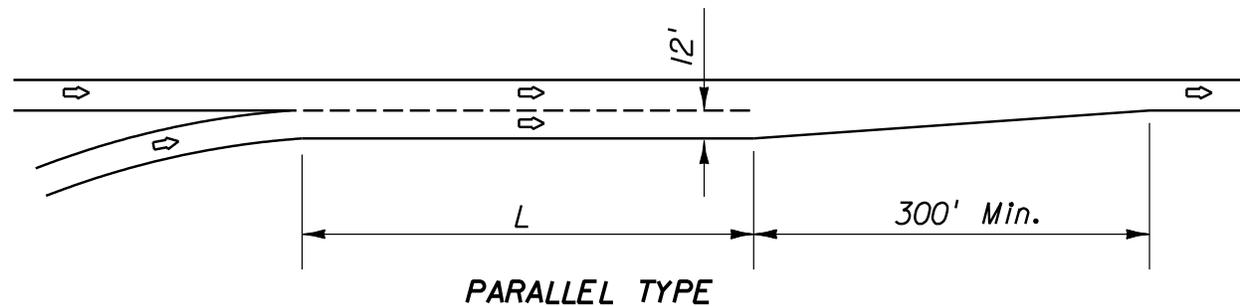
Recommended when design speed at entrance curve is less than 50 mph.
