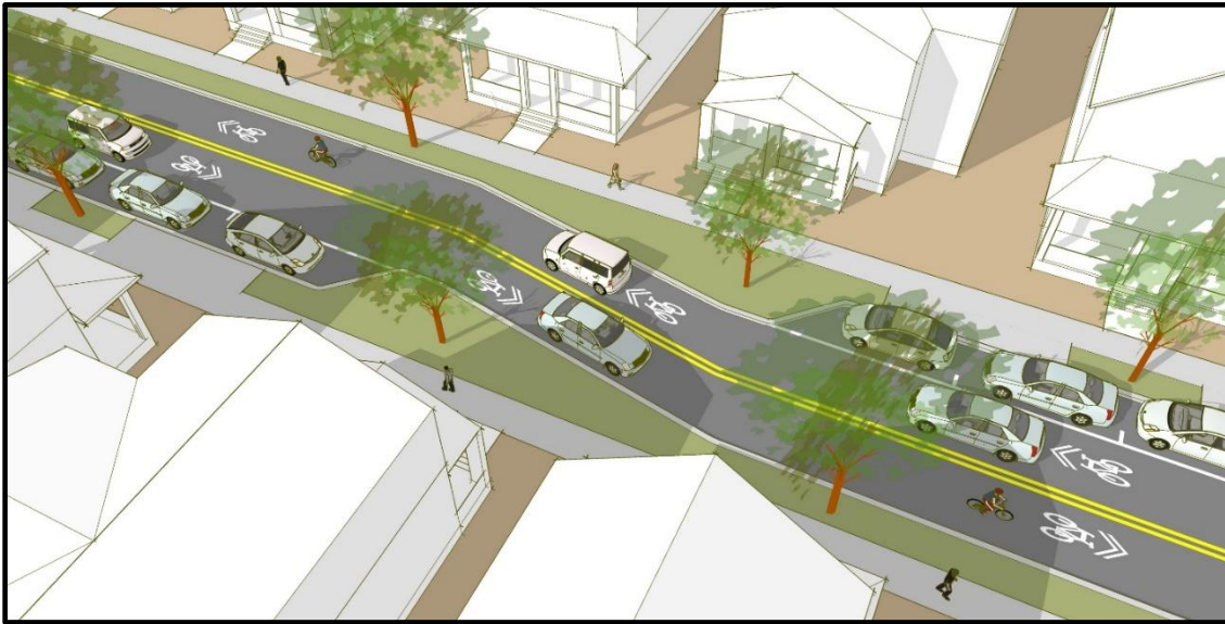
Figure 202.3.1 Concept Sketch - Midblock Chicane
