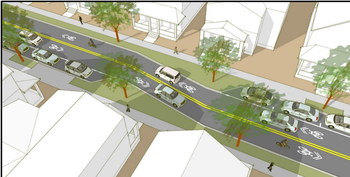
Figure 202.3.1 Concept Sketch - Midblock Chicane
