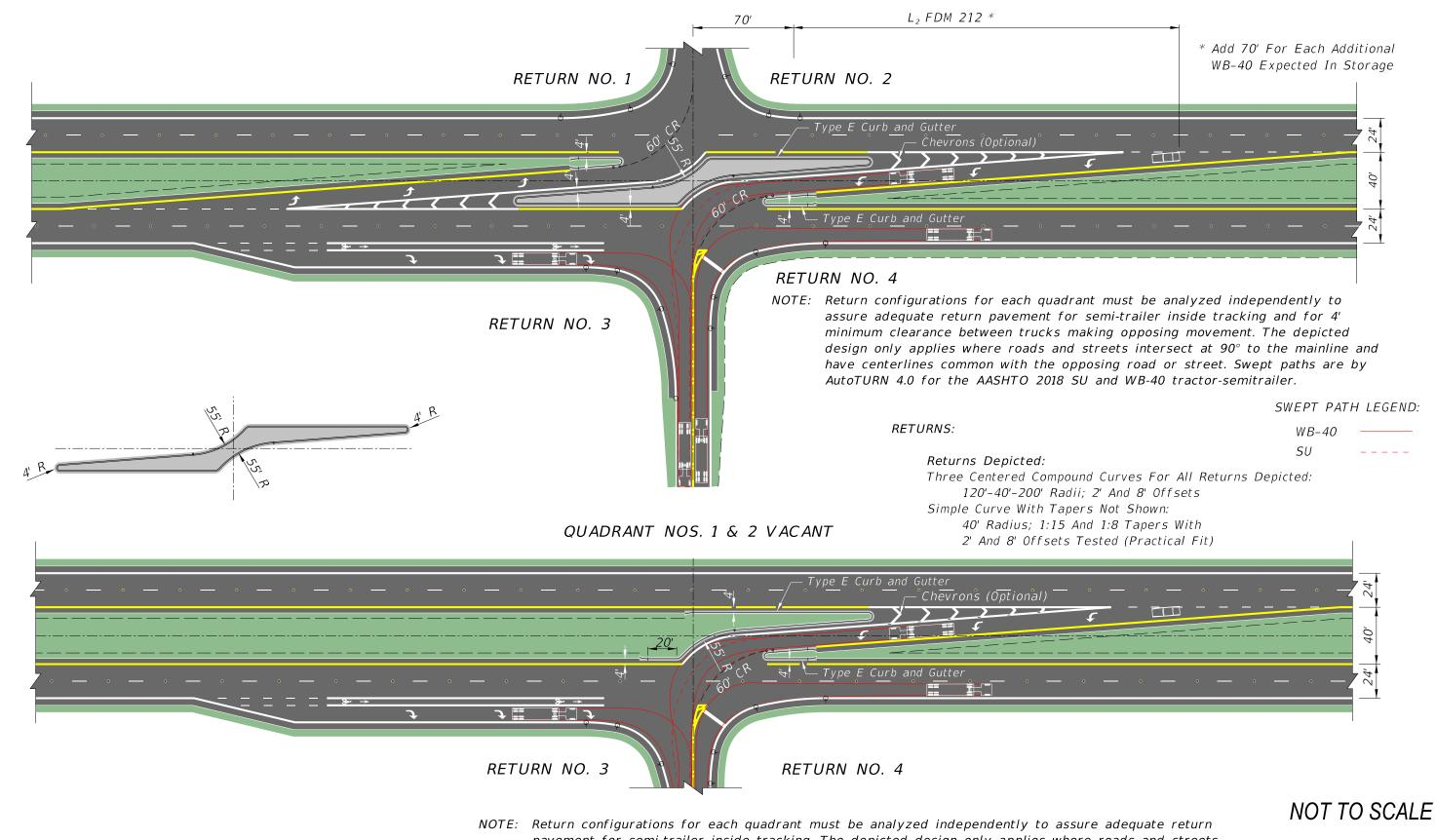
NOTE: Return configurations for each quadrant must be analyzed independently to assure adequate return pavement for semi-trailer inside tracking. The depicted design only applies where roads and streets intersect at 90° to the mainline. Swept paths are by AutoTURN 4.0 for the AASHTO 2018 SU and WB-40 tractor-semitrailer.
