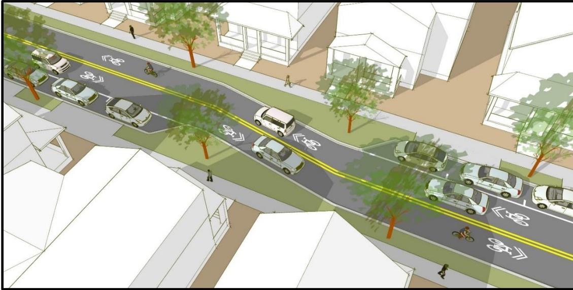
Figure 202.3.1 Concept Sketch - Midblock Chicane
