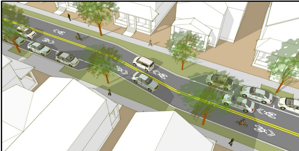
Figure 202.3.1 Concept Sketch - Midblock Chicane
