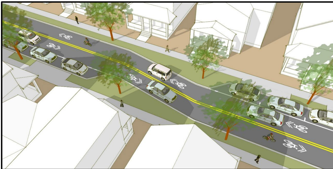
Figure 202.3.1 Concept Sketch - Midblock Chicane
