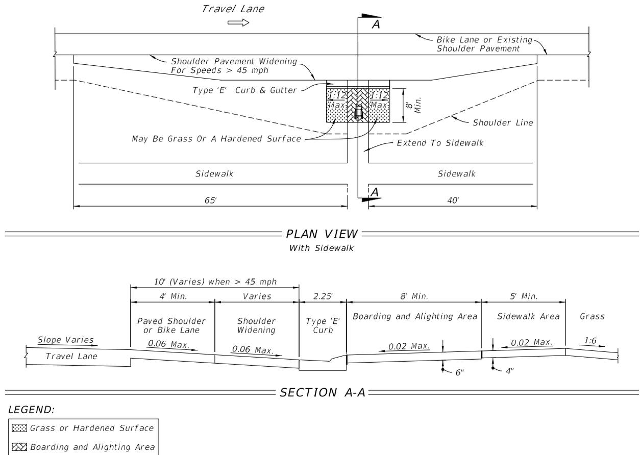
**Figure 225.2.2 Accessible Boarding and Alighting Area for Flush Shoulder Roadways with Connection to Roadway**
