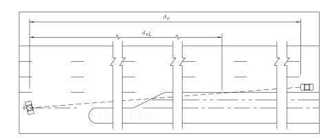
Where The Median Is Sufficiently Wide For The Design Vehicle To Pause In The Median (Vehicle d<sub>V</sub>) Is Measured From The Vehicle n; Distances d<sub>r</sub> & d<sub>m</sub> Do Not Apply.
