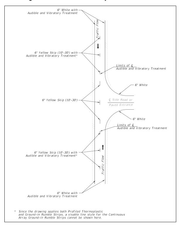
Figure 210.4.4 Audible and Vibratory Treatment Placement
