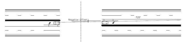
At locations where the full offset distances cannot be obtained, it is recommended that the minimum offset distances shown in **Table 212.14.1** be provided to achieve minimum required sight distances according to design speed. It is recommended that the "Opposing Truck" values be used where the opposing left-turn traffic includes a moderate to heavy volume of large trucks.
