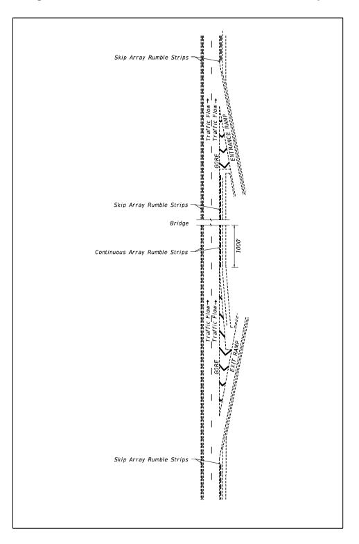
Figure 211.4.4 Placement of Ground-In Rumble Strips
