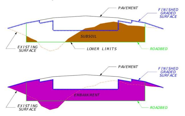
Figure 216.4.8 Excavation and Embankment
