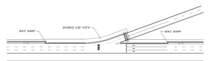
Figure 211.18.2 Example of Mitigation for Low-Angle Ramp
