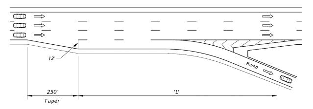
Figure 211.13.4 Parallel Design Type Exit Ramp Terminal
