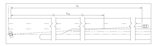
Where The Median Is Sufficiently Wide For The Design Vehicle To Pause In The Median (Vehicle Length Plus 6' Min.) The Clear Line Of Sight To The Right (d $_V$ ) Is Measured From The Vehicle Pause Location, i.e., Not From The Cross Road Stop Position; Distances  $d_r \& d_m$  Do Not Apply.
