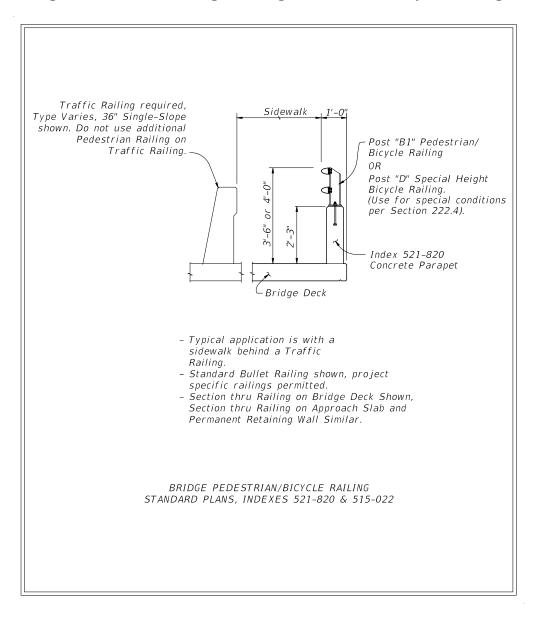
Figure 222.4.2 Bridge Railing – Pedestrian/Bicycle Railing
