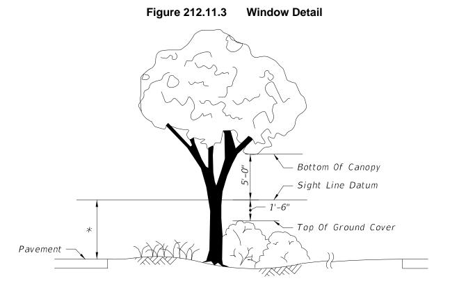
\* Since observations are made in both directions, the line-of-sight datum between roadways is 3.5 feet above both pavements.
