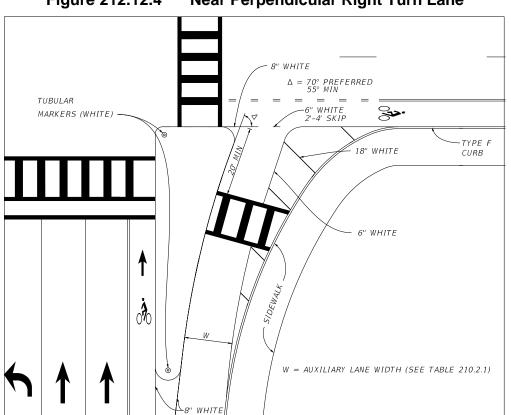
Figure 212.12.4 Near Perpendicular Right Turn Lane
