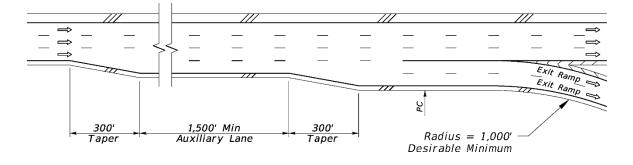
Figure 211.13.5 Two-Lane Parallel Design Type Exit Ramp Terminal
