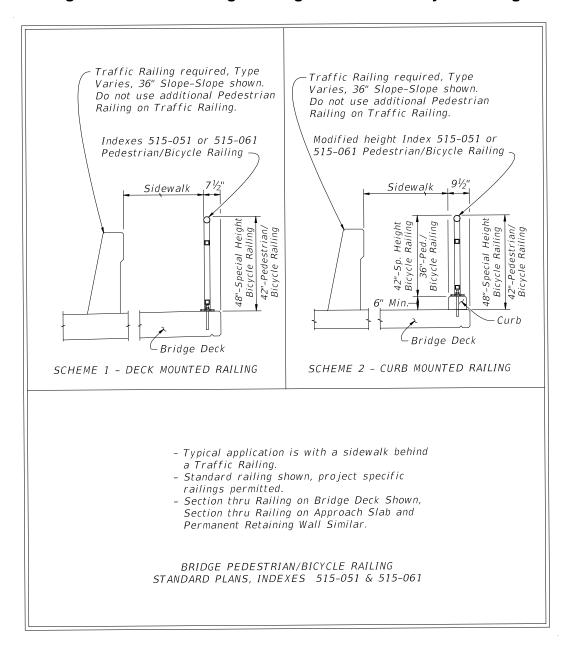
Figure 222.4.3 Bridge Railing – Pedestrian/Bicycle Railing
