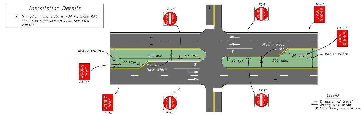
WRONG-WAY SIGNING AND PAVEMENT MARKING AT 3-LEG UNSIGNALIZED INTERSECTIONS ALONG DIVIDED ARTERIALS/COLLECTORS
