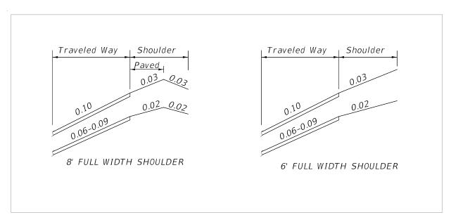
Figure 211.4.2 Special Ramp Shoulder Superelevation
