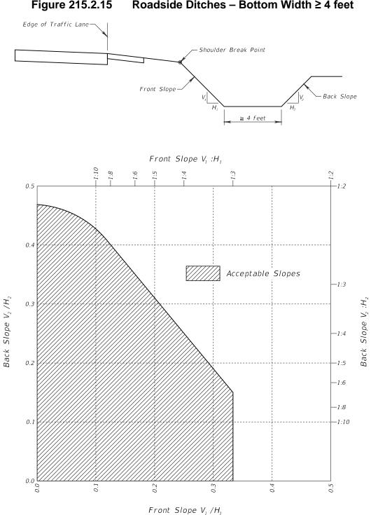
Figure 215.2.15 Roadside Ditches – Bottom Width ≥ 4 feet
