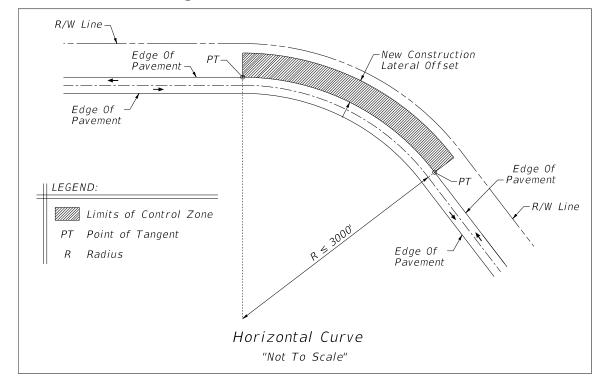
Figure 215.2.12 Horizontal Curve
