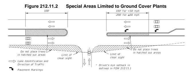
Where left turns from the major road are permitted, do not locate trees within the distance  $d_b$  shown in **Table 212.11.1** (see **FDM 212.11.4**) and not less than the distances shown in **Figure 212.11.2** and the spacings in **Table 212.11.3** as applicable.
