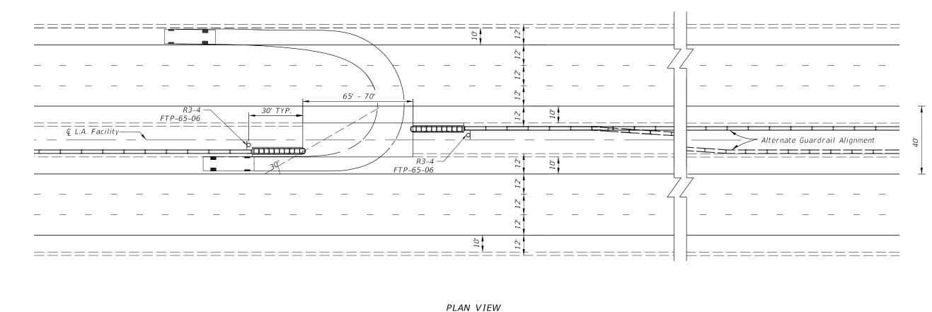
LEGEND: Crash Cushion 🛨 Barrier þ Sign SU Vehicle R3-4 (36"x36") OFFICIAL FTP-65-06 (36"×18") USE ONLY NOTES: 1. Provide Yellow RPMs placed outside yellow edge line in advance of crossover as shown in Standard Plans, Index 706-001. 2. Minimum turning radius for SU vehicle shown, and were generated by AutoTURN.
