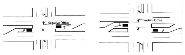
Figure 212.14.1 Negative and Positive Offset Left Turns
