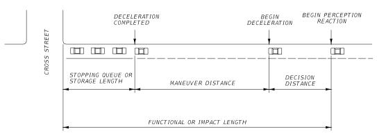
Figure 212.4.3 Elements of the Functional Area
