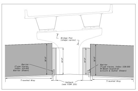
Figure 260.6.5 Curbed Roadway with Traffic Barrier
