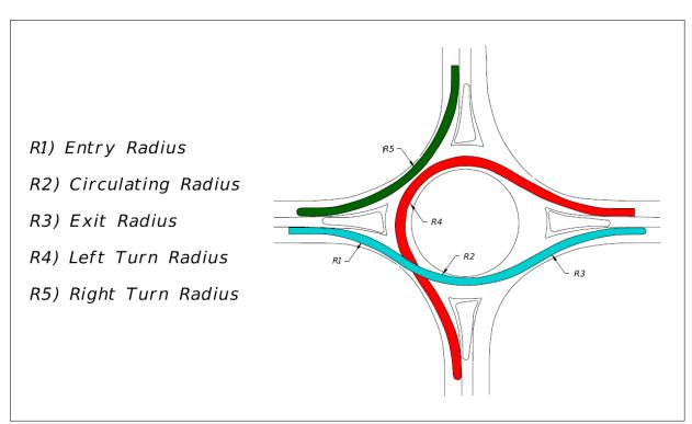
Figure 213.6.1 Fastest Path Curves
