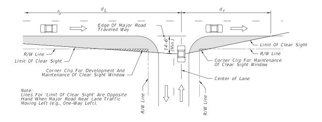
The minimum driver-eye setback of 14.5 feet from the edge of the traveled way may be adjusted on any intersection leg only when justified by a documented, site-specific field study of vehicle stopping position and driver-eye position.
