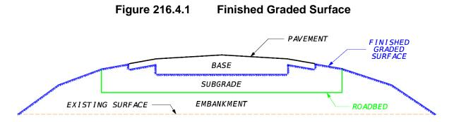
Projects are constructed over natural topography (Case I) or over existing roadbeds (Case II). Project may also have sections where both Case I and Case II apply.
