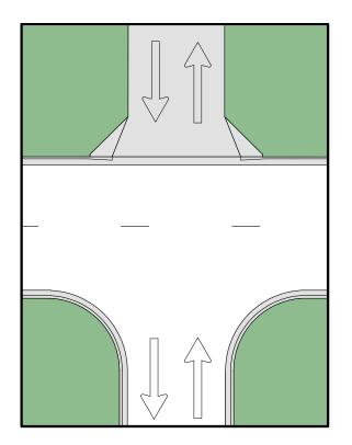
Figure 214.3.2 Aligned Through Lanes
