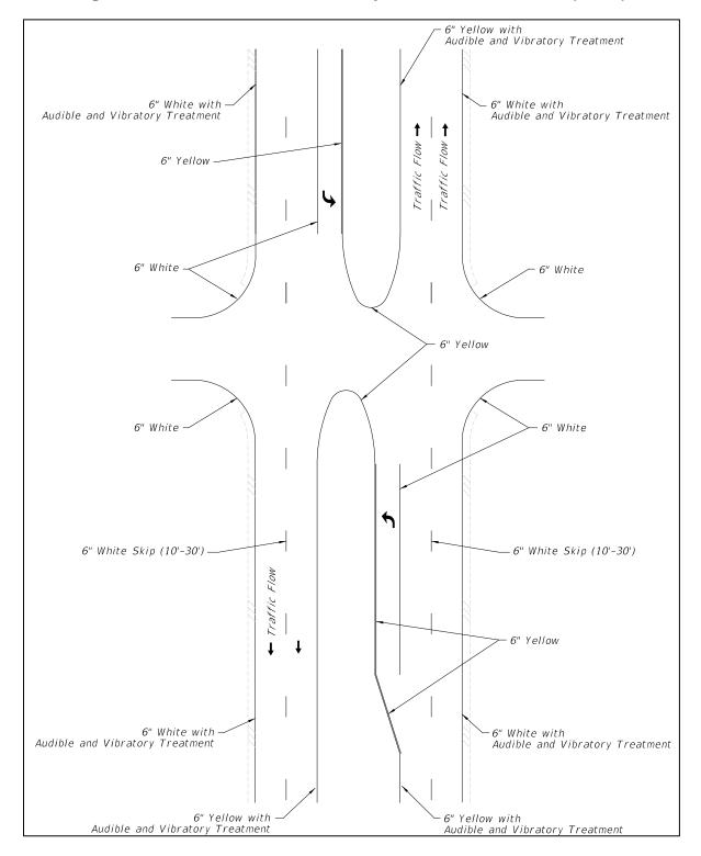
Figure 210.4.4 Audible and Vibratory Treatment Placement (Cont.)
