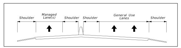
Figure 211.3.1 Managed Lanes Barrier Separation Typical Section
