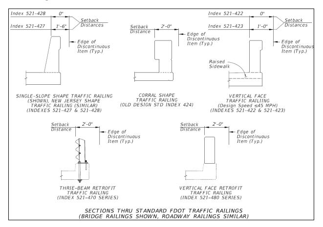
Figure 215.4.7 Setback Distances for Discontinuous Elements
