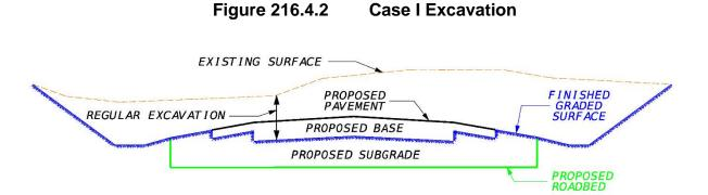
Calculate the Embankment quantities from the existing surface to the finished graded surface.
