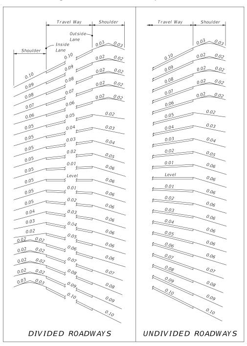
Figure 210.4.2 Shoulder Superelevation
