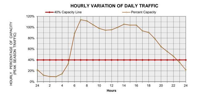
**<u>STEP 2</u>**: Identify the traffic pacing restrictions. Leave a buffer period of one hour between the end of traffic pacing operations and the beginning of 40% capacity.
