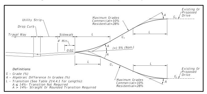
Figure 214.4.2 Curbed Roadway Driveway Profiles
