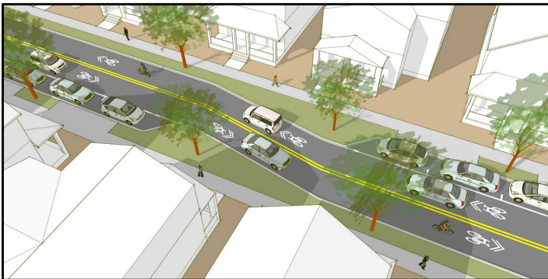
Figure 202.3.1 Concept Sketch - Midblock Chicane
