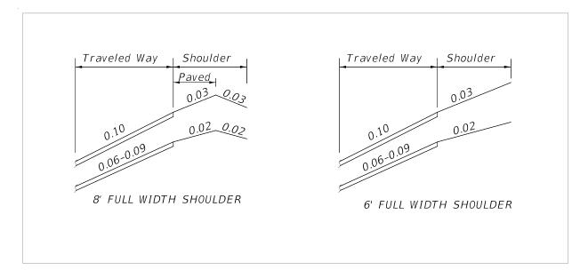
Figure 211.4.2 Special Ramp Shoulder Superelevation
