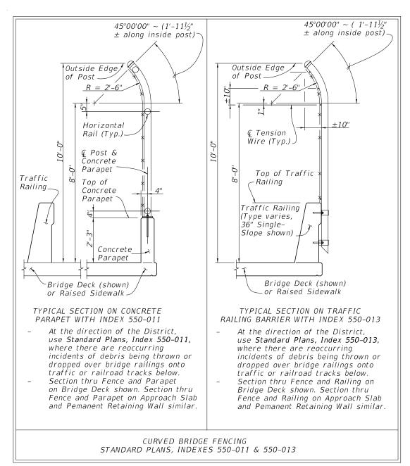
Figure 222.4.8 Bridge Railing – Enclosed Fencing
