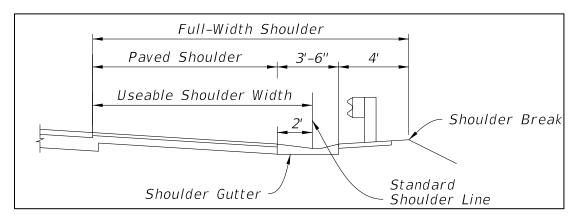
Figure 211.4.5 Useable Shoulder Width with Shoulder Gutter
