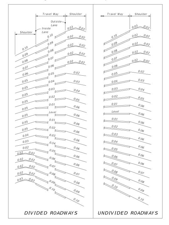
Figure 210.4.2 Shoulder Superelevation
