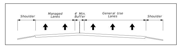
Figure 211.3.3 Managed Lanes Wide Buffer Separation Typical Section
