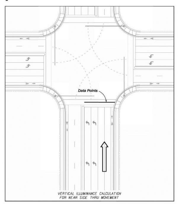
Figure 231.3.2 Vertical Illuminance Calculation for Right Turn Approach
