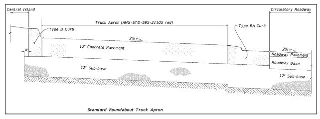
Figure 213.3.2 Standard Truck Apron Design
