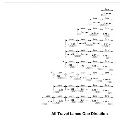
Figure 210.2.1 Standard Pavement Cross Slopes
