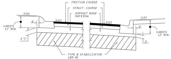
DETAIL OF ASPHALT BASE CURB PAD
