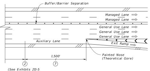
Single-Lane Ramp with Auxiliary Lane Configuration
