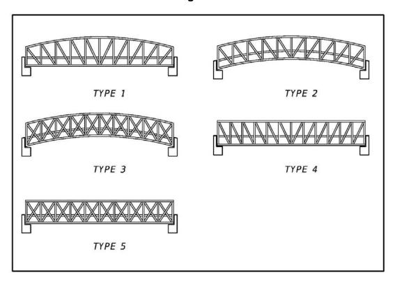
Figure 266.4.3 Prefabricated Pedestrian Bridge Standard Truss Member Shapes
