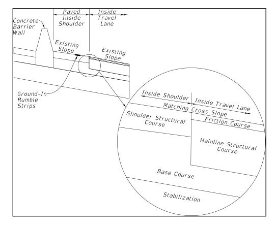
Figure 211.4.3 Flush Shoulder Pavement
