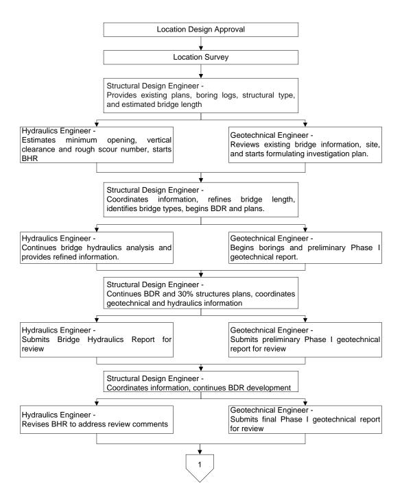
Figure 250.2.1 Structural Plans Development
