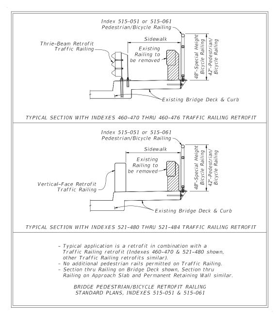
Figure 222.4.6 Bridge Railing and Bridge Parapet Fencing
