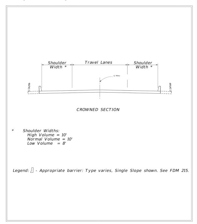
Figure 260.1.3 Partial Bridge Sections for Curbed Arterials and Collectors
