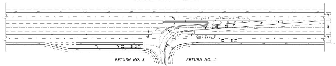
NOTE: Return configurations for each quadrant must be analyzed independently to assure adequate return pavement for semi-trailer inside tracking. The depicted design only applies where roads and streets intersect at 90° to the mainline. Swept paths are by AutoTURN 4.0 for the AASHTO 2018 SU and WB-40 tractor-semitrailer.
