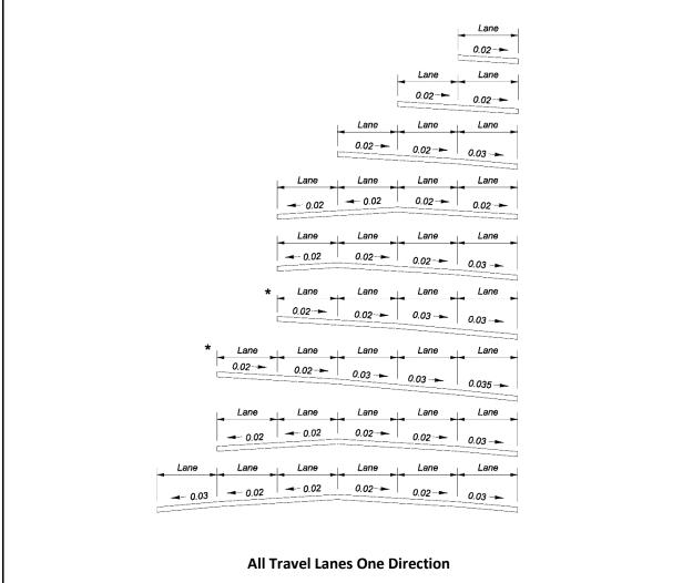
Figure 211.2.1 Standard Pavement Cross Slopes
