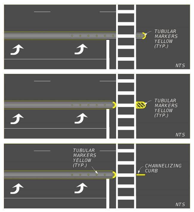
Figure 210.3.7 Hardened Centerline without Traffic Separator
