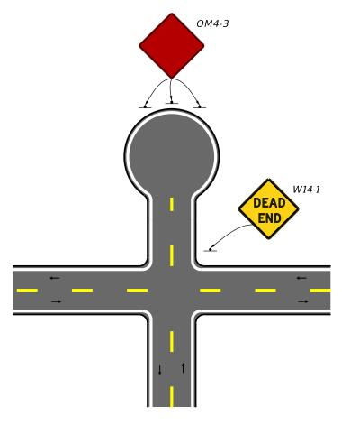
Figure 2 TRAFFIC CONTROLS FOR CUL-DE-SAC OR DEAD END
