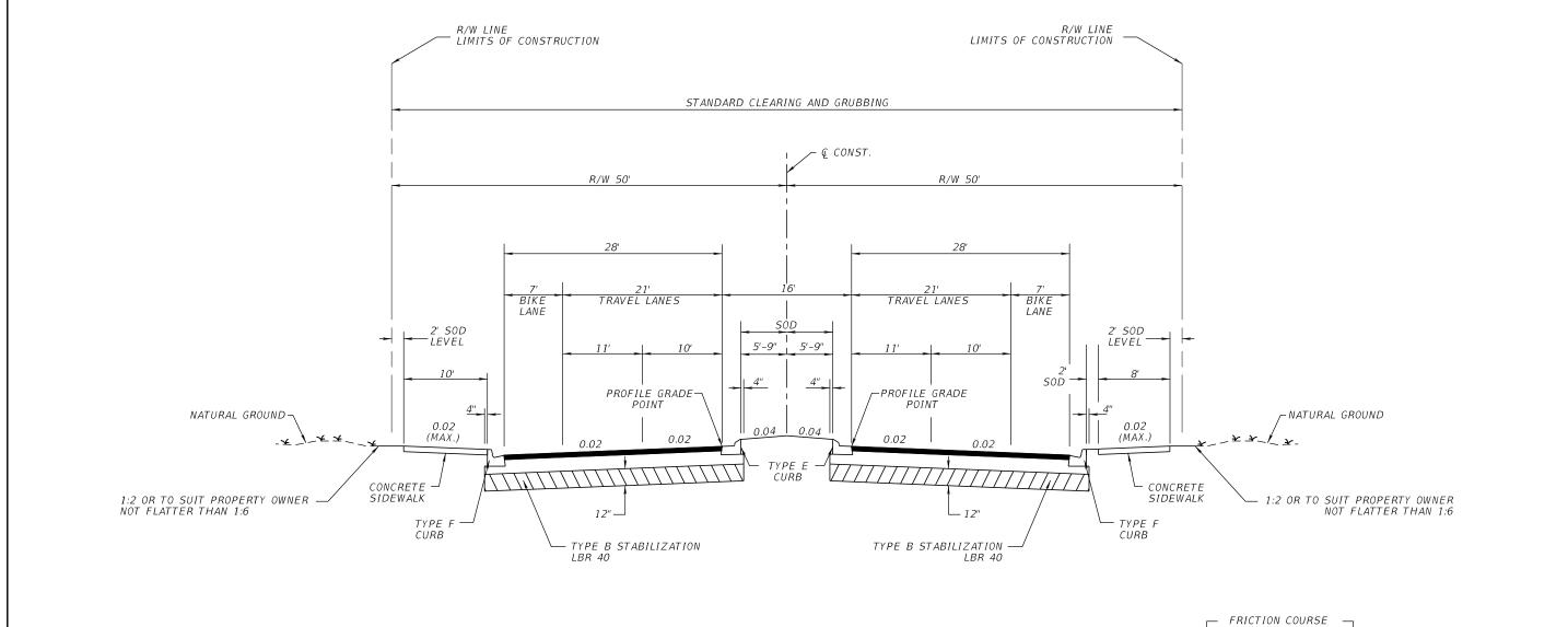
CURRENT YEAR = 2018 AADT = 22800 ESTIMATED OPENING YEAR = 2020 AADT = 25800 ESTIMATED DESIGN YEAR = 2040 AADT = 30600 K = 6% D = 55% T = 2% (24 HOUR) DESIGN HOUR T = 1% DESIGN SPEED = 30 MPH CONTEXT CLASSIFICATION = C2T TYPICAL SECTION
