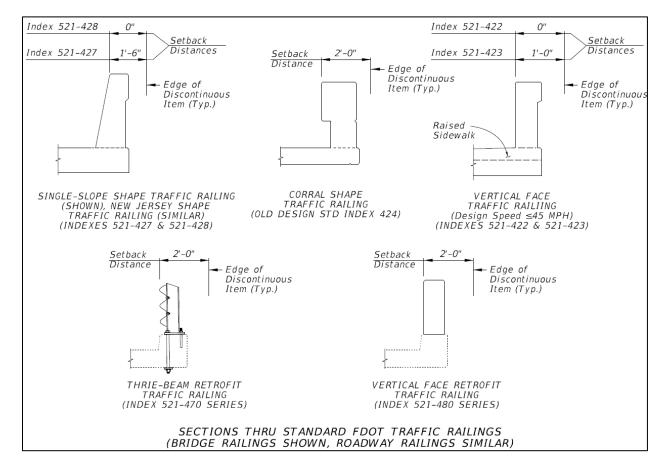
Figure 215.4.7 Setback Distances for Discontinuous Elements
