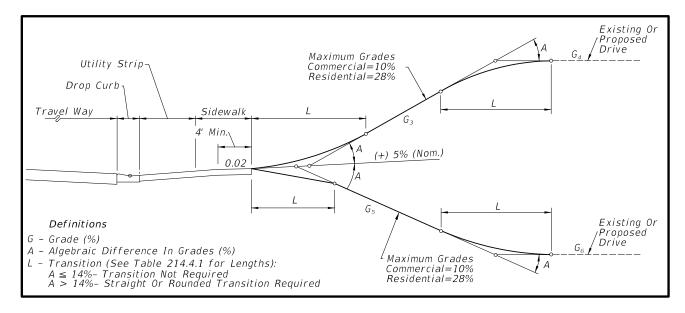
Figure 214.4.2 Curbed Roadway Driveway Profiles
