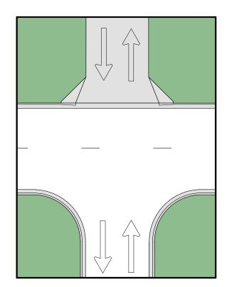
Figure 214.3.2 Aligned Through Lanes
