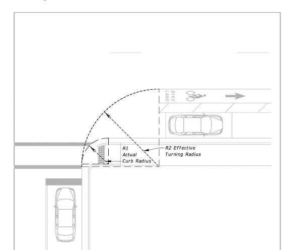
Figure 212.12.2 Actual Curb Radius Vs Effective Radius
