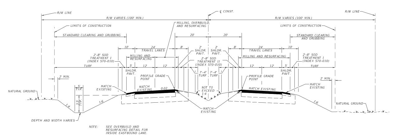
CURRENT YEAR = 2018 AADT = 18100 ESTIMATED OPENING YEAR = 2020 AADT = 21000 ESTIMATED DESIGN YEAR = 2036 AADT = 38900 K = 11% D = 58% T = 22% (24 HOUR) DESIGN HOUR T = 11% DESIGN SPEED = 60 MPH POSTED SPEED = 55 MPH CONTEXT CLASSIFICATION = C2 ESURFACING DETAIL FUR ISIDE EASTBOUND LANE.
