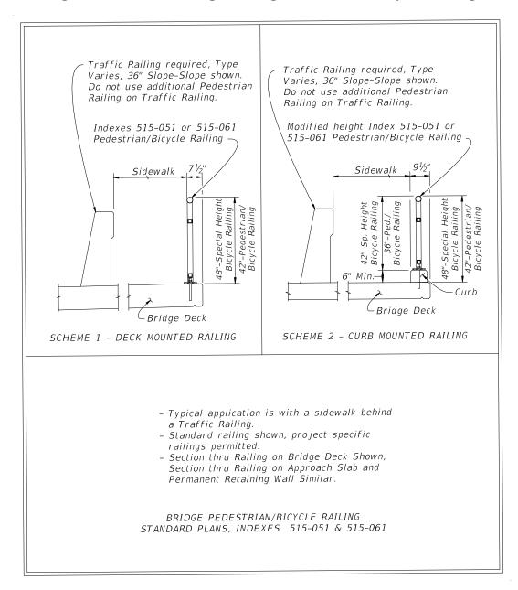
Figure 222.4.4 Bridge Railing – Pedestrian/Bicycle Railing
