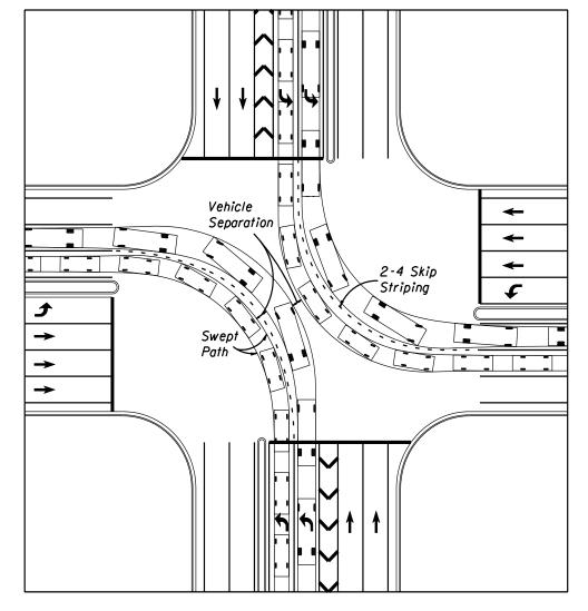
Figure 212.12.6 P and SU Design Vehicles Turning Simultaneously
