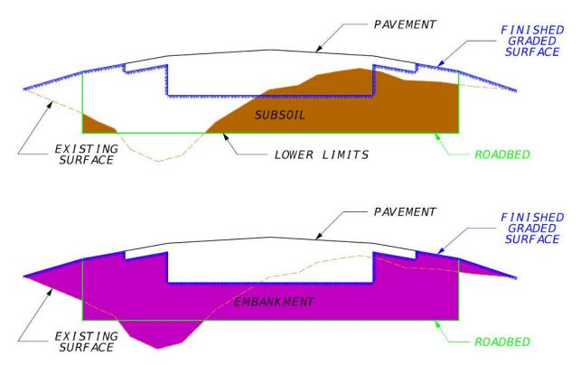
Figure 216.4.8 Excavation and Embankment
