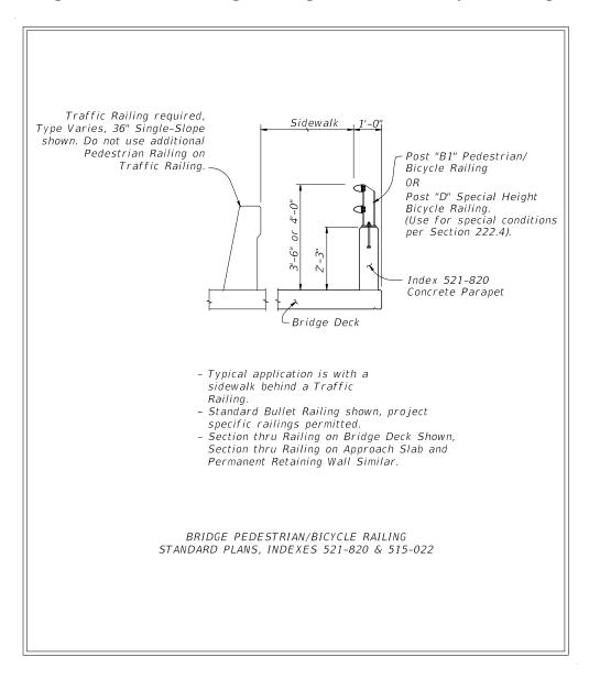
Figure 222.4.3 Bridge Railing – Pedestrian/Bicycle Railing
