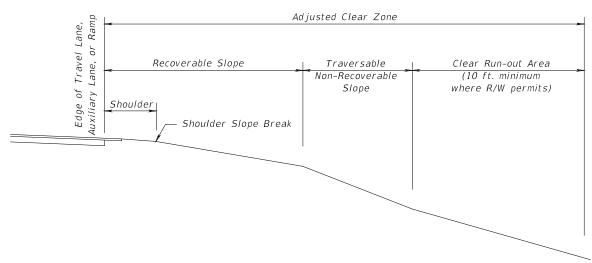
Figure 215.2.3 Adjusted Clear Zone Concept
