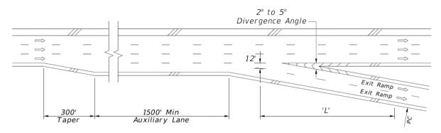
Figure 211.13.3 Two-Lane Taper Type Exit Ramp Terminal
