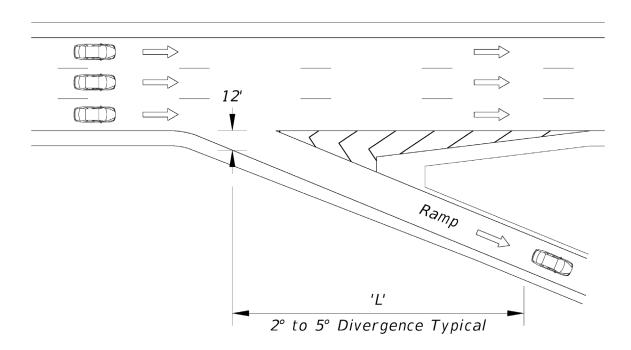
Figure 211.13.2 Taper Type Exit Ramp Terminal
