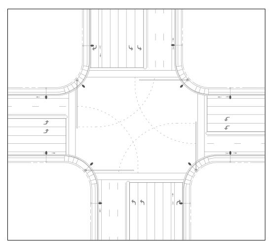
Figure 231.3.4 Typical Lighting Layout for Large Intersection
