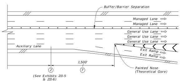
Two-Lane Ramp with Auxiliary Lane Configuration
