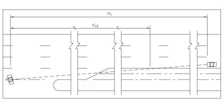
Where The Median Is Sufficiently Wide For The Design Vehicle To Pause In The Median (Vehicle Length Plus 6' Min.) The Clear Line Of Sight To The Right (d $_{
