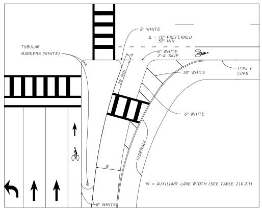
Figure 212.12.4 Near Perpendicular Right Turn Lane
