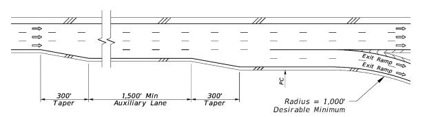
Figure 211.13.5 Two-Lane Parallel Design Type Exit Ramp Terminal
