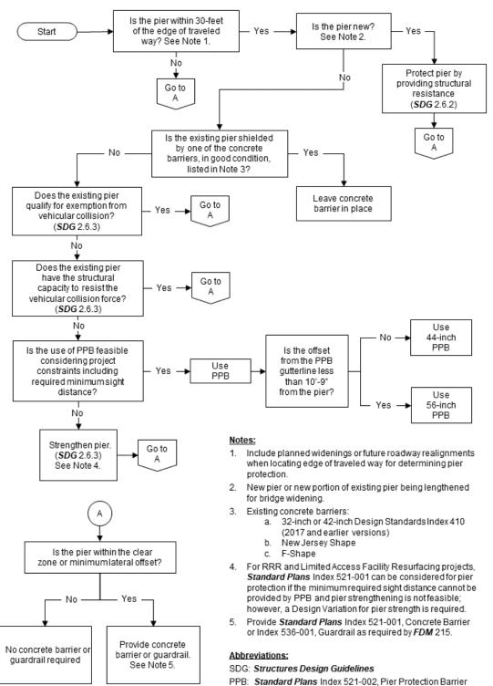
Figure 215.4.5 Pier Protection Selection Flowchart
