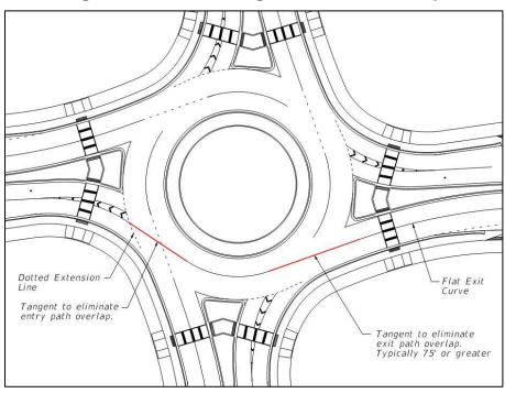
Figure 213.4.1 Tangents for Path Overlap
