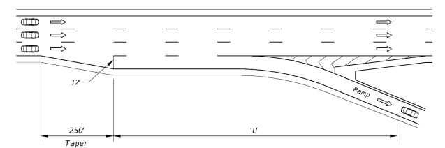
Figure 211.13.4 Parallel Design Type Exit Ramp Terminal
