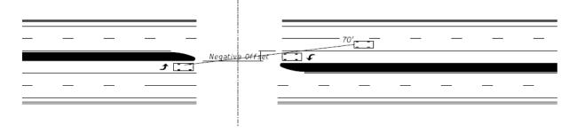
On curbed roadway designs, offset left-turn lanes should be used with median widths greater than 18 feet. A 4-foot traffic separator should be used when possible to channelize the left turn and provide separation from opposing traffic.
