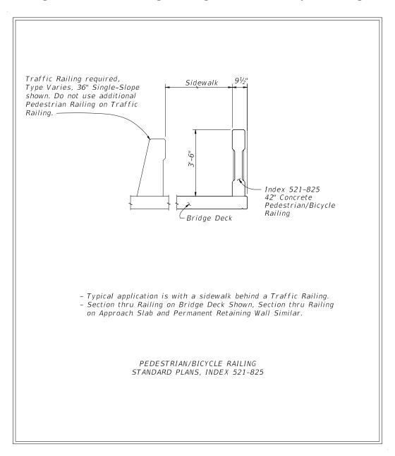
Figure 222.4.5 Bridge Railing and Pedestrian/Bicycle Railing Retrofit
