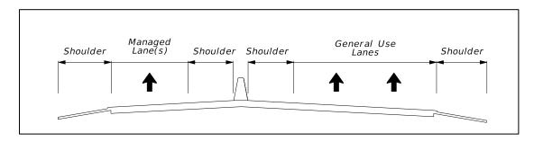
Figure 211.3.2 Managed Lanes Buffer Separation with Tubular Marker Typical Section
