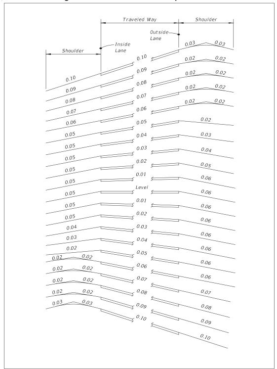
Figure 211.4.1 Shoulder Superelevation
