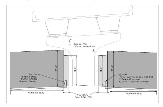
Figure 260.6.5 Curbed Roadway with Traffic Barrier
