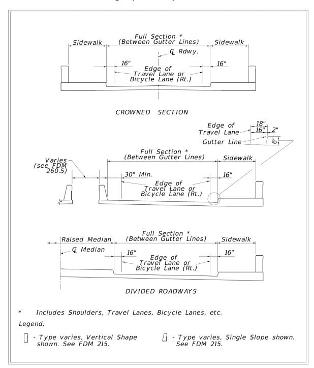
Figure 260.1.4 Bridge Section for Divided Arterials and Collectors
