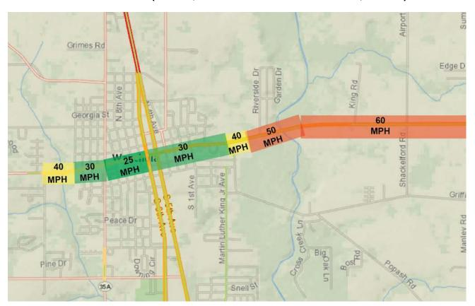
Figure 202.4.4 Section Change Near Transition from 40 to 30 mph (Entrance to Wauchula, FL, showing lane narrowing)
