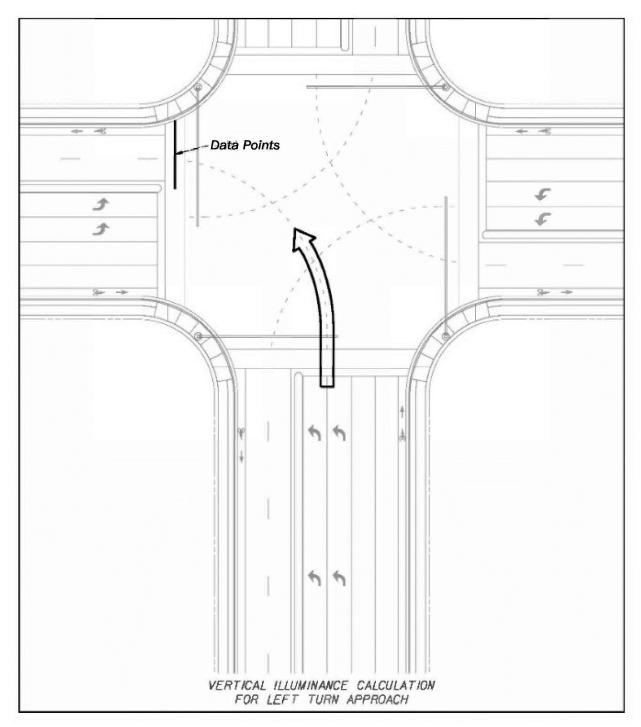
*Figure 231.3.4* shows the typical lighting layout for a large intersection. The crosswalk and luminaire locations must be coordinated to optimize the vertical illumination level.
