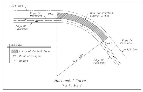
Figure 215.2.12 Horizontal Curve
