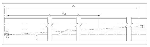
Where The Median Is Sufficiently Wide For The Design Vehicle To Pause In The Median (Vehicle Length Plus 6' Min.) The Clear Line Of Sight To The Right ( $d_V$ ) Is Measured From The Vehicle Pause Location, i.e., Not From The Cross Road Stop Position; Distances  $d_r \& d_m$  Do Not Apply.
