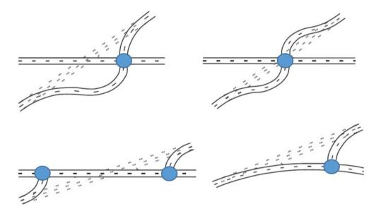
Figure 213.3.1 Realignment Configurations
