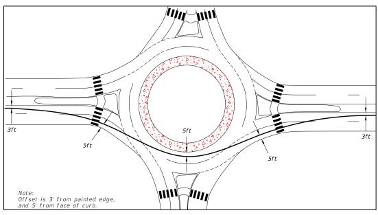
Figure 213.6.3 Fastest Path for Right Turn Movement
