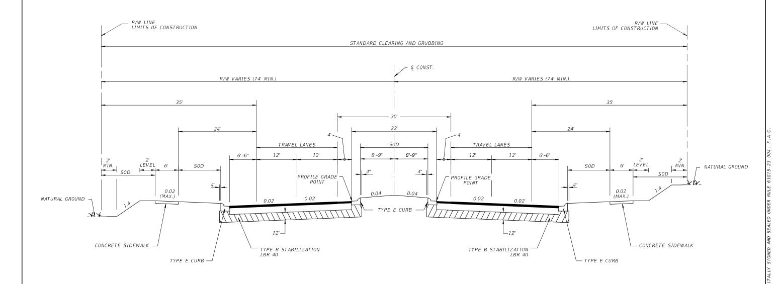
CURRENT YEAR = 2018 AADT = 22800 ESTIMATED OPENING YEAR = 2020 AADT = 25800 ESTIMATED DESIGN YEAR = 2040 AADT = 30600 K = 6% D = 55% T = 2% (24 HOUR) DESIGN HOUR T = 1% DESIGN SPEED = 50 MPH CONTEXT CLASSIFICATION = C3 TYPICAL SECTION
