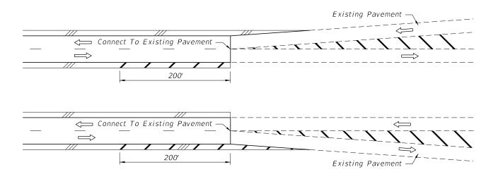
CONNECTING ROADWAY WITH PAVED SHOULDERS TO EXISTING ASYMMETRICAL FLARE WITHOUT PAVED SHOULDERS
