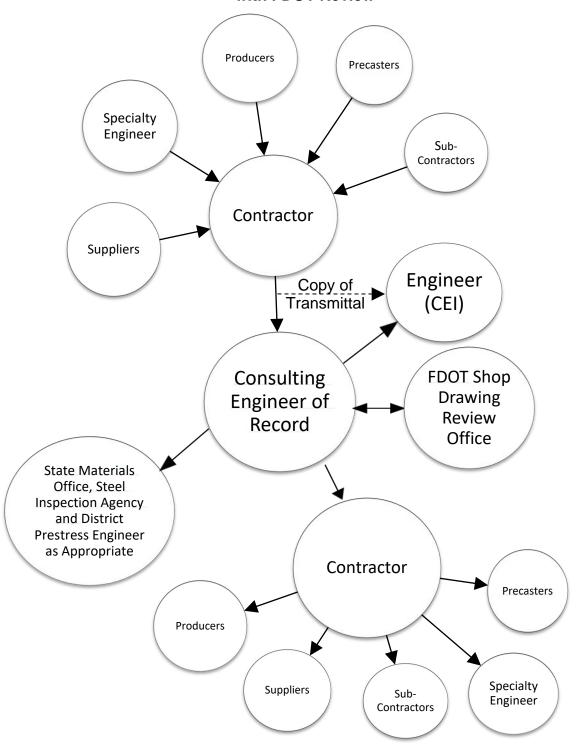
Figure 152.11.3 Shop Drawing Flow Diagram for Reviews Performed by FDOT Only
