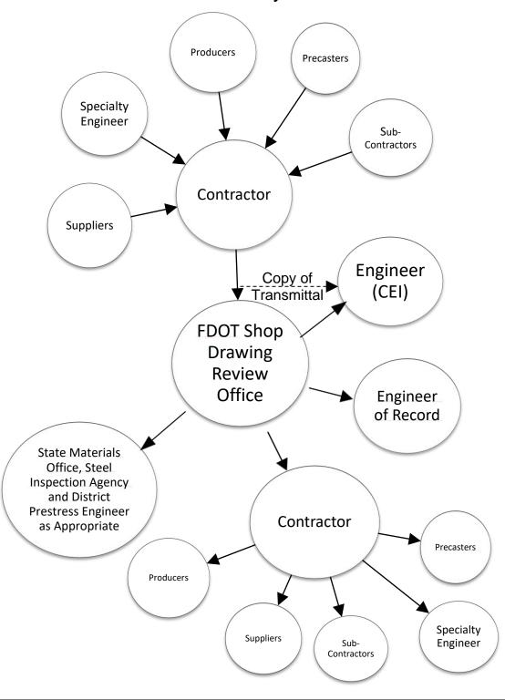
Figure 152.11.4 Shop Drawing Flow Diagram for Design-Build Project- Shop Drawings Affecting Public Safety
