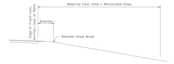
When a Traversable Non-Recoverable Slope is present within the clear zone, extend the clear zone width until the amount of Recoverable Slope equals the required clear zone width obtained from *Table 215.2.1*. The additional width provided beyond the Traversable Non-Recoverable Slope is known as the Clear Run-out Area and is illustrated in *Figure 215.2.3*. Provide a 10-foot minimum width for the Clear Run-out Area where R/W allows.
