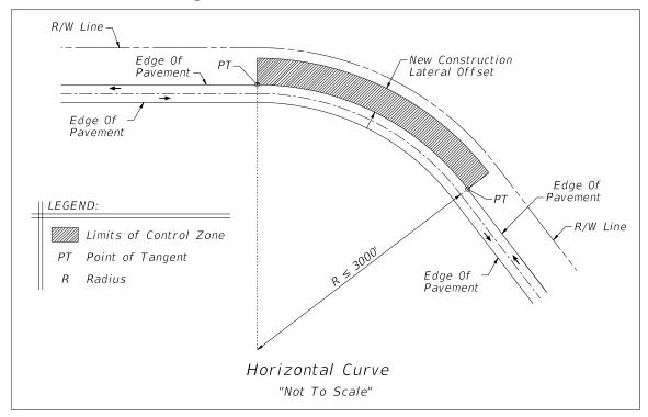
Figure 215.2.12 Horizontal Curve
