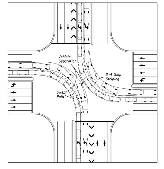
Figure 212.12.5 P and SU Design Vehicles Turning Simultaneously
