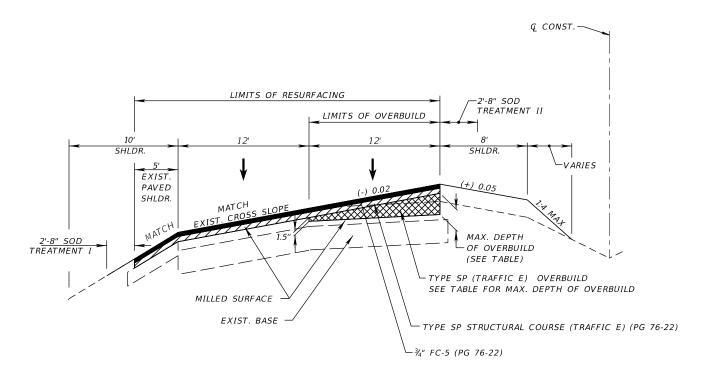
OVERBUILD AND RESURFACING DETAIL
