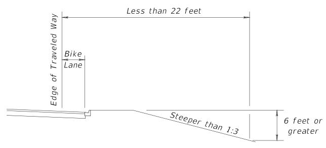
Figure 215.3.3 Drop-off Hazard on Low-Speed Curbed Roadways
