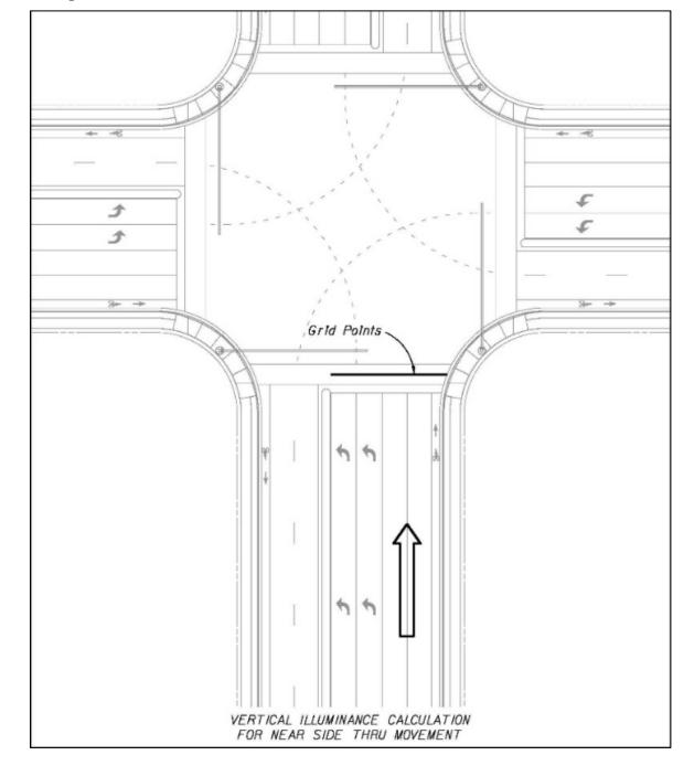
Figure 231.3.1 Vertical Illuminance Calculation for Near Side Movement
