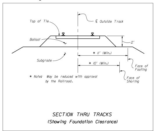
Figure 220.3.2 Section Thru Tracks
