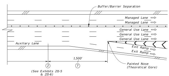
Two-Lane Ramp with Auxiliary Lane Configuration
