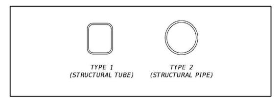
Figure 266.3.3 Prefabricated Pedestrian Standard Bridge Cross-Sections
