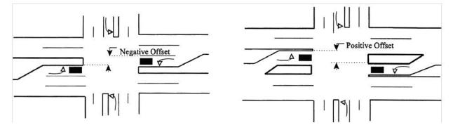
The conventional method of designing left turn lanes is to place the left turn lanes adjacent to the through lanes. This design creates a negative offset which restricts the sight distance of the left-turning driver's view of oncoming traffic when another vehicle is in the opposing turn lane. *Figure 212.14.2* indicates the negative offset when the conventional design is used.
