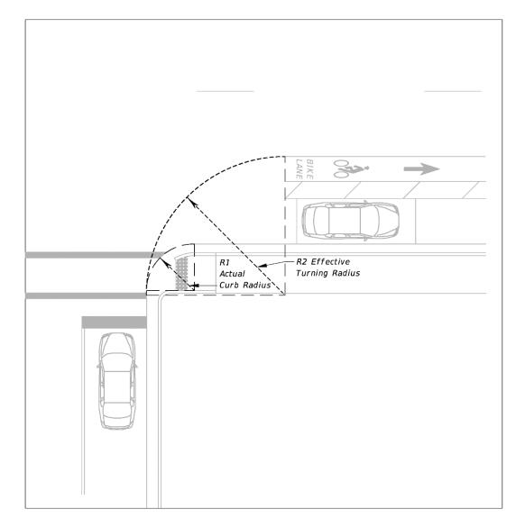
Figure 212.12.2 Actual Curb Radius Vs Effective Radius
