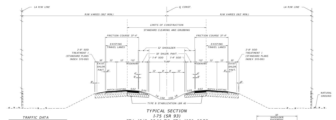
= 2018 AADT = 22300ESTIMATED OPENING YEAR = 2020 AADT = 23300 ESTIMATED DESIGN YEAR = 2040 AADT = 51500 K = 9 % D = 56 % T = 10 % (24 HOUR)DESIGN HOUR T = 5 %DESIGN SPEED = 70 MPH CONTEXT CLASSIFICATION = N/A
