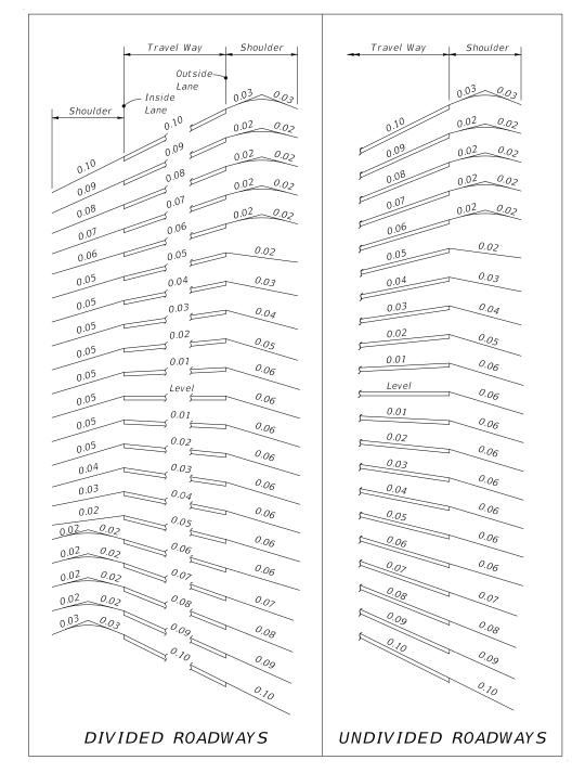
Figure 210.4.2 Shoulder Superelevation
