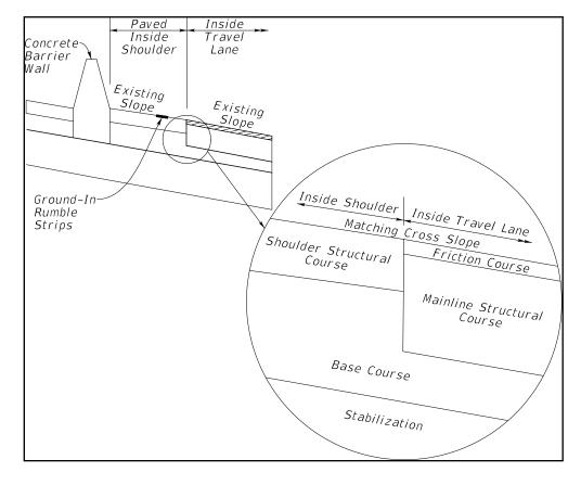
Figure 211.4.3 Flush Shoulder Pavement
