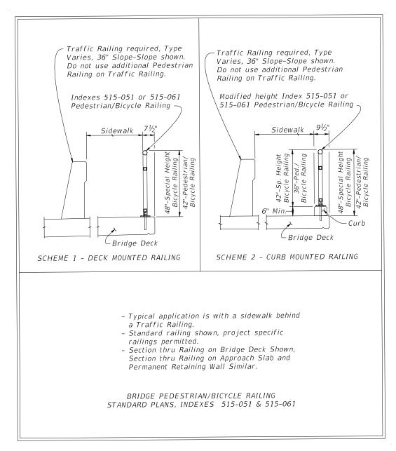
Figure 222.4.4 Bridge Railing – Pedestrian/Bicycle Railing
