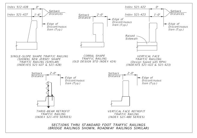
Figure 215.4.7 Setback Distances for Discontinuous Elements
