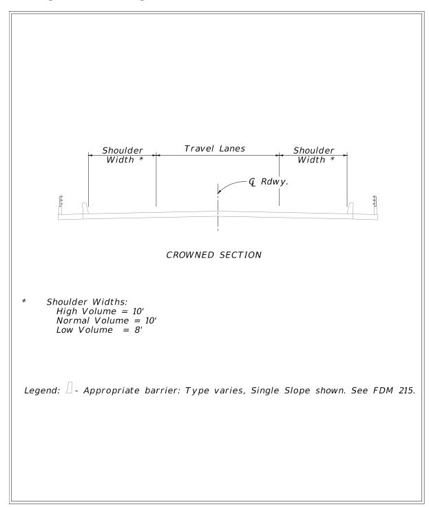
Figure 260.1.3 Partial Bridge Sections for Curbed Arterials and Collectors
