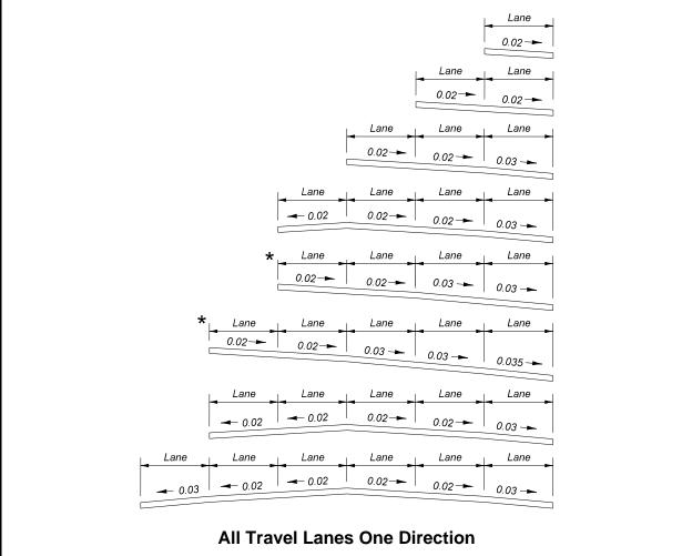
Figure 211.2.1 Standard Pavement Cross Slopes
