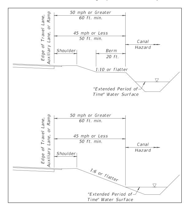
Figure 215.3.2 Lateral Offset Criteria for Canal Hazards on Curbed Roadways
