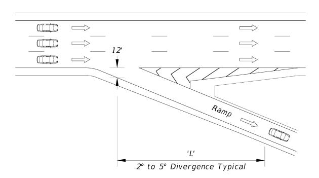
Figure 211.13.2 Taper Type Exit Ramp Terminal
