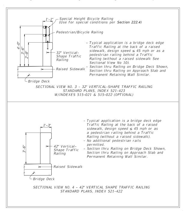
Figure 215.4.3 Bridge Traffic Railings – Other Shapes
