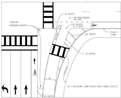
Figure 212.12.4 Near Perpendicular Right Turn Lane
