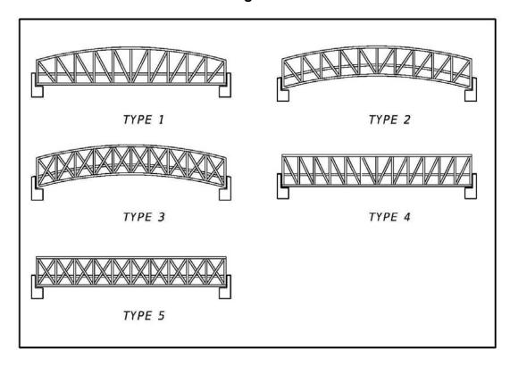
Figure 266.3.2 Prefabricated Pedestrian Bridge Standard Truss Member Shapes
