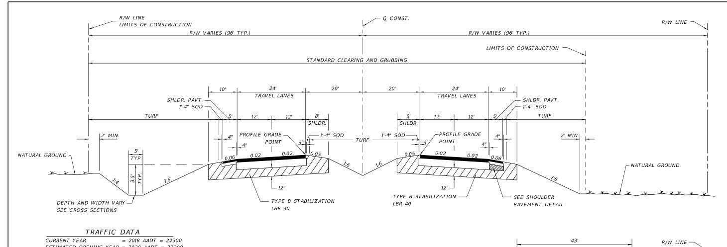
CURRENT YEAR = 2018 AADT = 22300 ESTIMATED OPENING YEAR = 2020 AADT = 23300 ESTIMATED DESIGN YEAR = 2040 AADT = 51500 K = 9% D = 56% T = 10% (24 HOUR) DESIGN HOUR T = 5% DESIGN SPEED = 55 MPH CONTEXT CLASSIFICATION = C1
