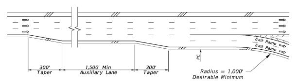
Figure 211.13.5 Two-Lane Parallel Design Type Exit Ramp Terminal
