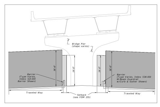
Figure 260.6.5 Curbed Roadway with Traffic Barrier
