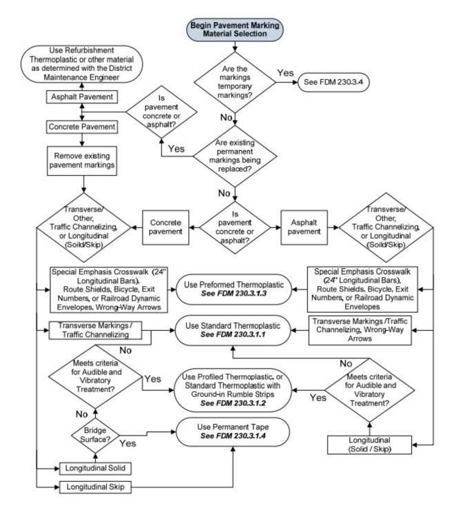
Figure 230.3.1 Pavement Marking Material Selection
