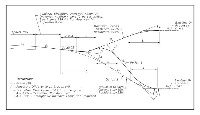
Figure 214.4.4 Driveway Slope for Flush Shoulder Roadway in Superelevation
