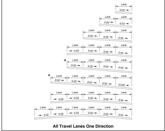
Figure 210.2.1 Standard Pavement Cross Slopes
