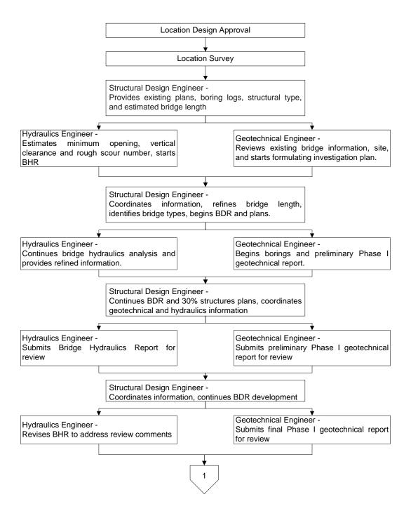
Figure 250.2.1 Structural Plans Development
