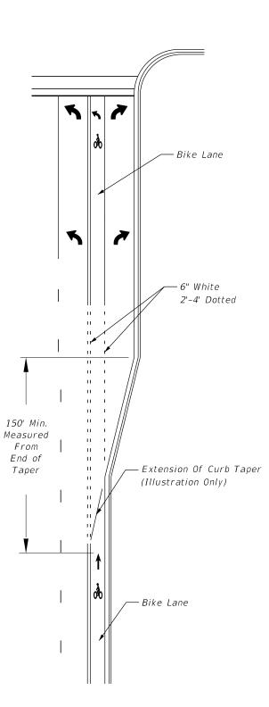
CURBED ROADWAY "TEE" INTERSECTION WITH SEPARATE RIGHT-TURN LANE
