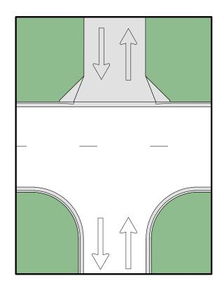
Figure 214.3.2 Aligned Through Lanes
