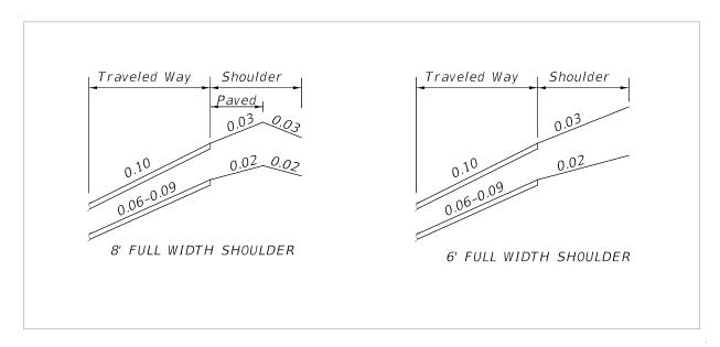
Figure 211.4.2 Special Ramp Shoulder Superelevation
