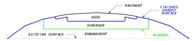
Projects are constructed over natural topography (Case I) or over existing roadbeds (Case II). Project may also have sections where both Case I and Case II apply.
