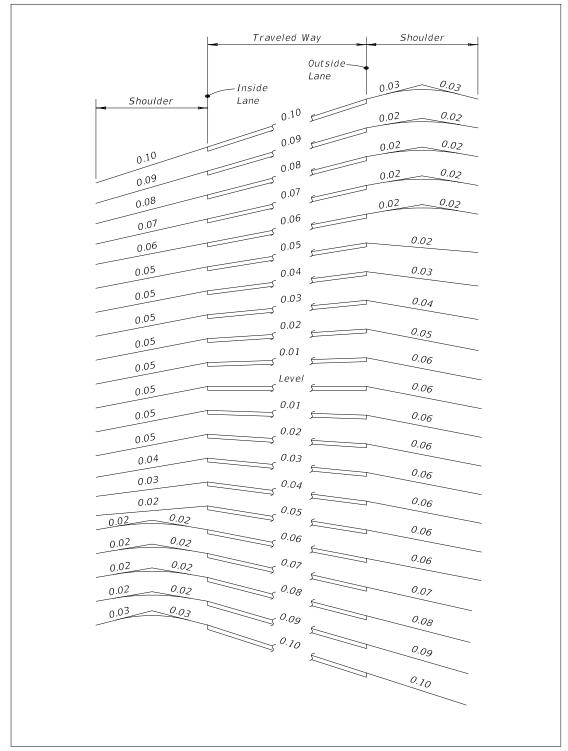
Figure 211.4.1 Shoulder Superelevation
