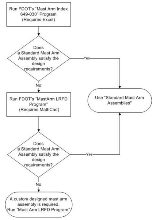
Figure 261.4.1 Flowchart for Designing Mast Arm Assemblies
