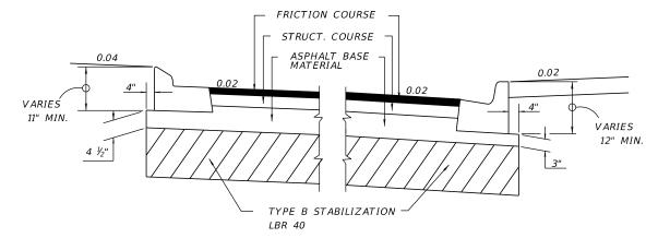
DETAIL OF ASPHALT BASE CURB PAD
