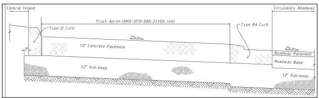
Figure 213.3.2 Standard Truck Apron Design
