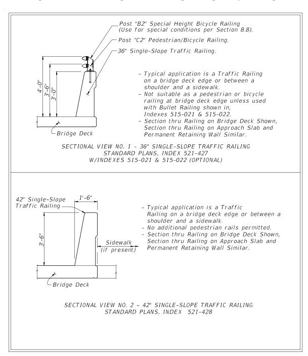
Figure 215.4.2 Bridge Traffic Railings – Vertical Shapes
