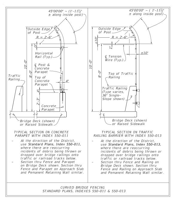
Figure 222.4.8 Bridge Railing – Enclosed Fencing
