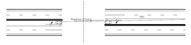
At locations where the full offset distances cannot be obtained, it is recommended that the minimum offset distances shown in *Table 212.14.1* be provided to achieve minimum required sight distances according to design speed. It is recommended that the "Opposing Truck" values be used where the opposing left-turn traffic includes a moderate to heavy volume of large trucks.
