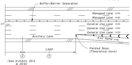
Single-Lane Ramp with Auxiliary Lane Configuration
