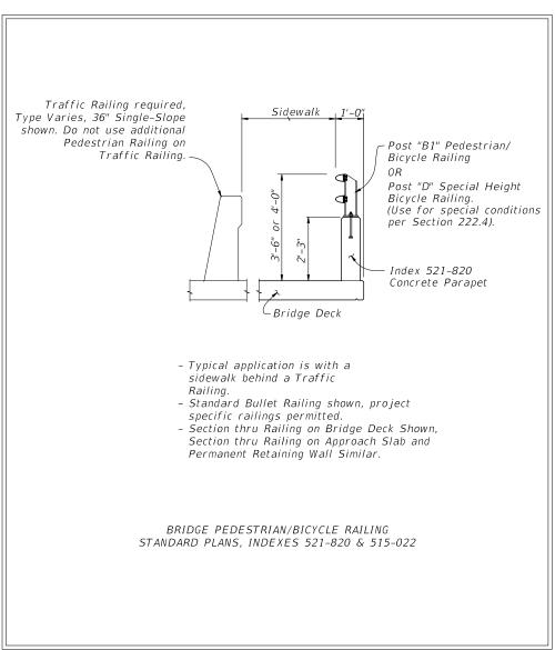
Figure 222.4.3 Bridge Railing – Pedestrian/Bicycle Railing
