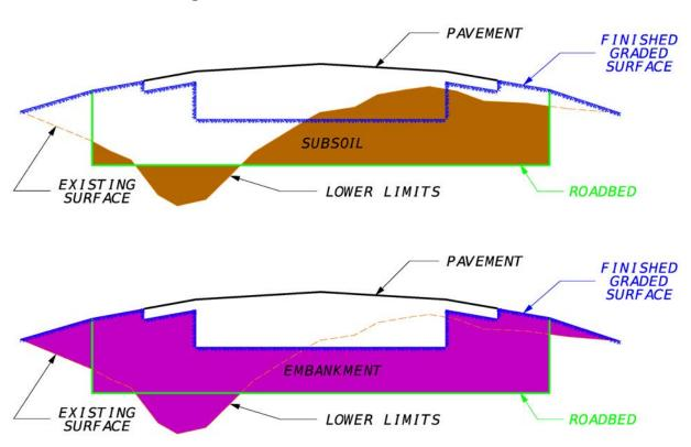
Figure 216.4.8 Excavation and Embankment
