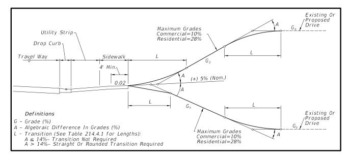
Figure 214.4.2 Curbed Roadway Driveway Profiles
