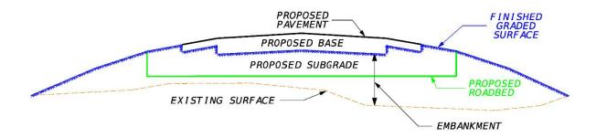
Case II projects may or may not include the removal of existing base material or removal of existing concrete pavement. According to **Standard Specification 120-4.2**:
