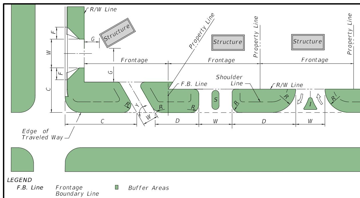
**Radius (R)** – The radial dimension of curved driveway entry or exit
