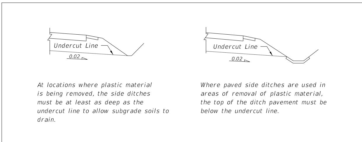
**Figure 216.4.8 Excavation and Embankment**
