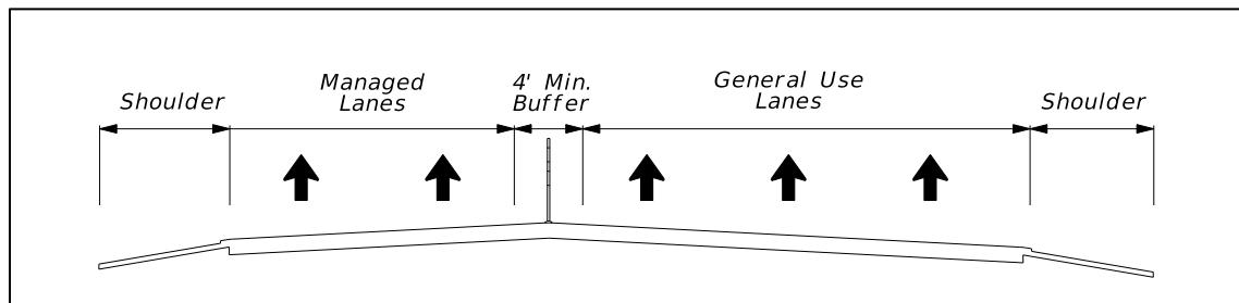
**Figure 211.3.3 Managed Lanes Wide Buffer Separation Typical Section**
