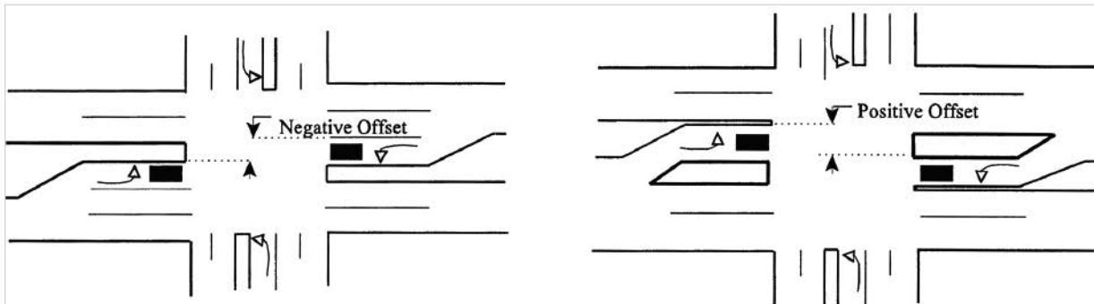
The conventional method of designing left turn lanes is to place the left turn lanes adjacent to the through lanes. This design creates a negative offset which restricts the sight distance of the left-turning driver's view of oncoming traffic when another vehicle is in the opposing turn lane. **Figure 212.14.2** indicates the negative offset when the conventional design is used.
