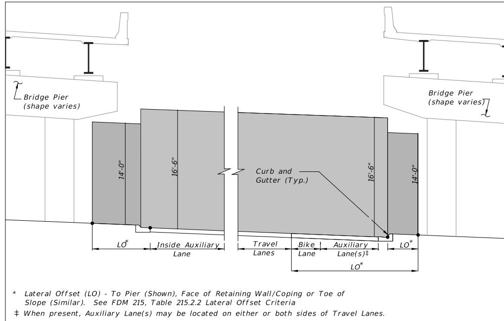
**Figure 260.6.5 Curbed Roadway with Traffic Barrier**
