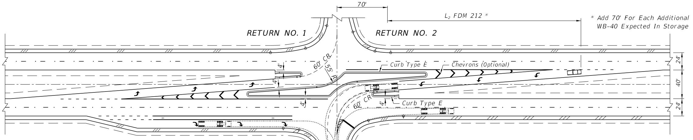
**NOTE:** Return configurations for each quadrant must be analyzed independently to assure adequate return pavement for semi-trailer inside tracking and for 4' minimum clearance between trucks making opposing movement. The depicted design only applies where roads and streets intersect at 90° to the mainline and have centerlines common with the opposing road or street. Swept paths are by AutoTURN 4.0 for the AASHTO 2001 SU and WB-40 tractor-semitrailer.
