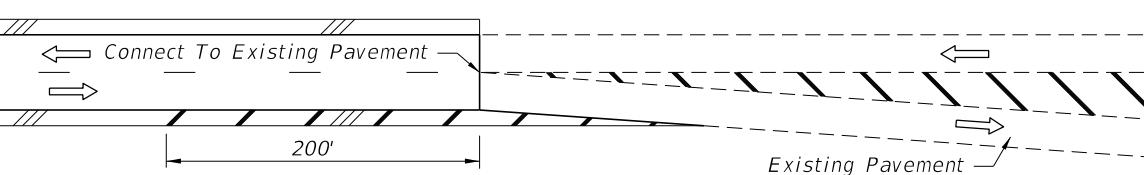
CONNECTING ROADWAY WITH PAVED SHOULDERS TO EXISTING ASYMMETRICAL FLARE WITHOUT PAVED SHOULDERS
