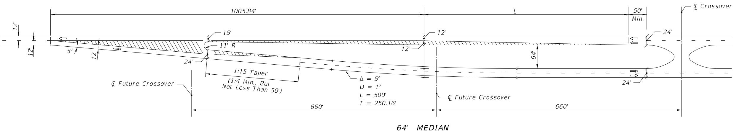
$$L = \frac{WS^2}{60} \quad \text{FOR DESIGN SPEEDS} \leq 40 \text{ mph}$$
