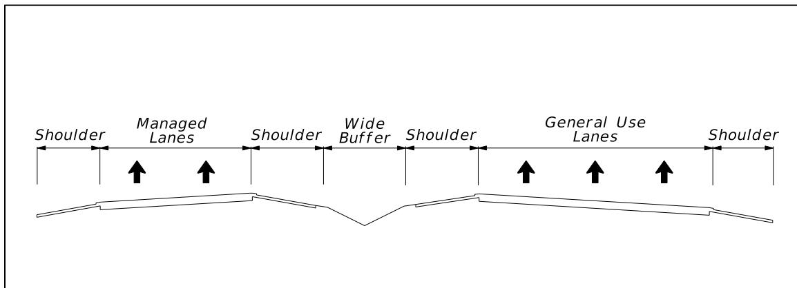
**Figure 211.3.4 Managed Lanes Grade Separation Typical Section**
