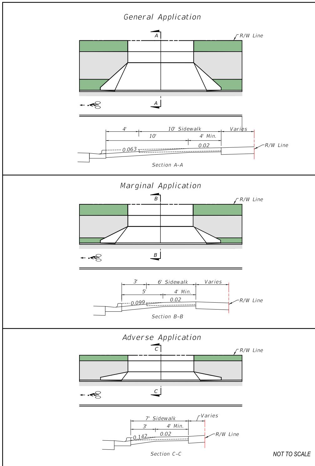
**Figure 214.4.2 Curbed Roadway Driveway Profiles**
