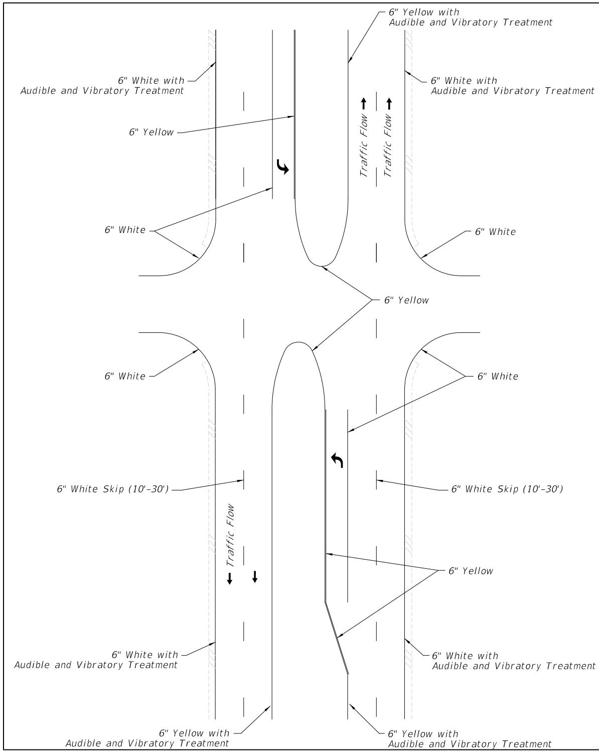
**Figure 210.4.4 Audible and Vibratory Treatment Placement (Cont.)**
