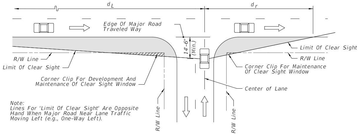
The minimum driver-eye setback of 14.5 feet from the edge of the traveled way may be adjusted on any intersection leg only when justified by a documented, site-specific field study of vehicle stopping position and driver-eye position.
