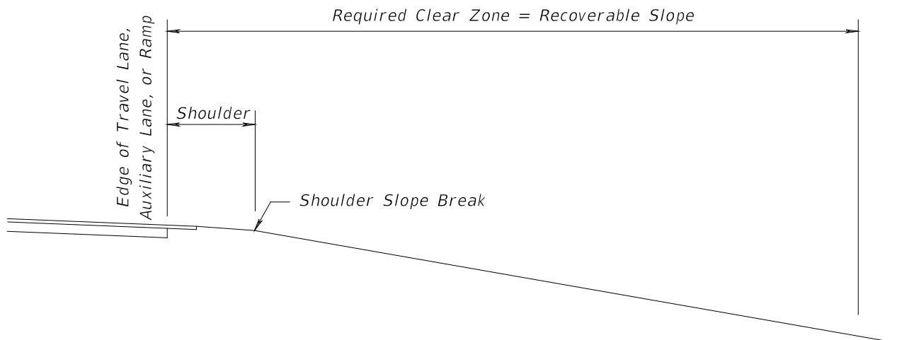
When a Traversable Non-Recoverable Slope is present within the clear zone, extend the clear zone width until the amount of Recoverable Slope equals the required clear zone width obtained from **Table 215.2.1**. The additional width provided beyond the Traversable Non-Recoverable Slope is known as the Clear Run-out Area and is illustrated in **Figure 215.2.3**. Provide a 10-foot minimum width for the Clear Run-out Area where R/W allows.
