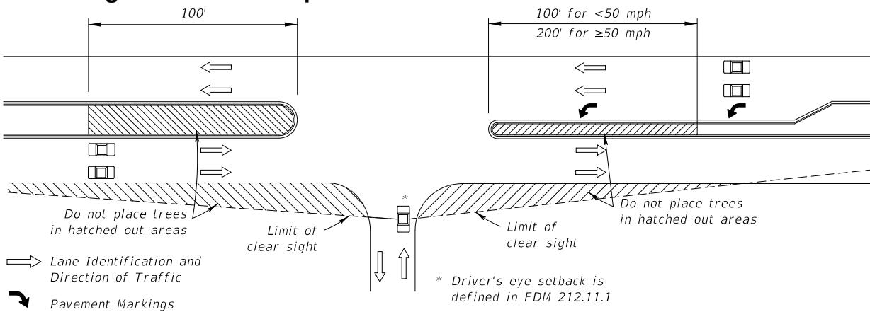
Where left turns from the major road are permitted, do not locate trees within the distance  $d_b$  shown in **Table 212.11.1** (see **FDM 212.11.4**) and not less than the distances shown in **Figure 212.11.2** and the spacings in **Table 212.11.3** as applicable.
