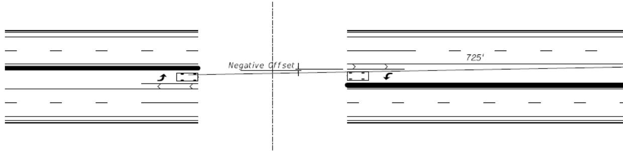
At locations where the full offset distances cannot be obtained, it is recommended that the minimum offset distances shown in **Table 212.14.1** be provided to achieve minimum required sight distances according to design speed. It is recommended that the "Opposing Truck" values be used where the opposing left-turn traffic includes a moderate to heavy volume of large trucks.
