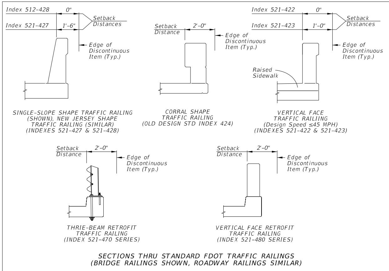
Noise Wall/Traffic Railing combinations located within the setback distance must be crash tested to or accepted as TL-4 under **MASH**. Other continuous items (e.g., glare screens and fences) located within this setback distance must be crash tested to or accepted as TL-3 under **NCHRP 350** or **MASH**.
