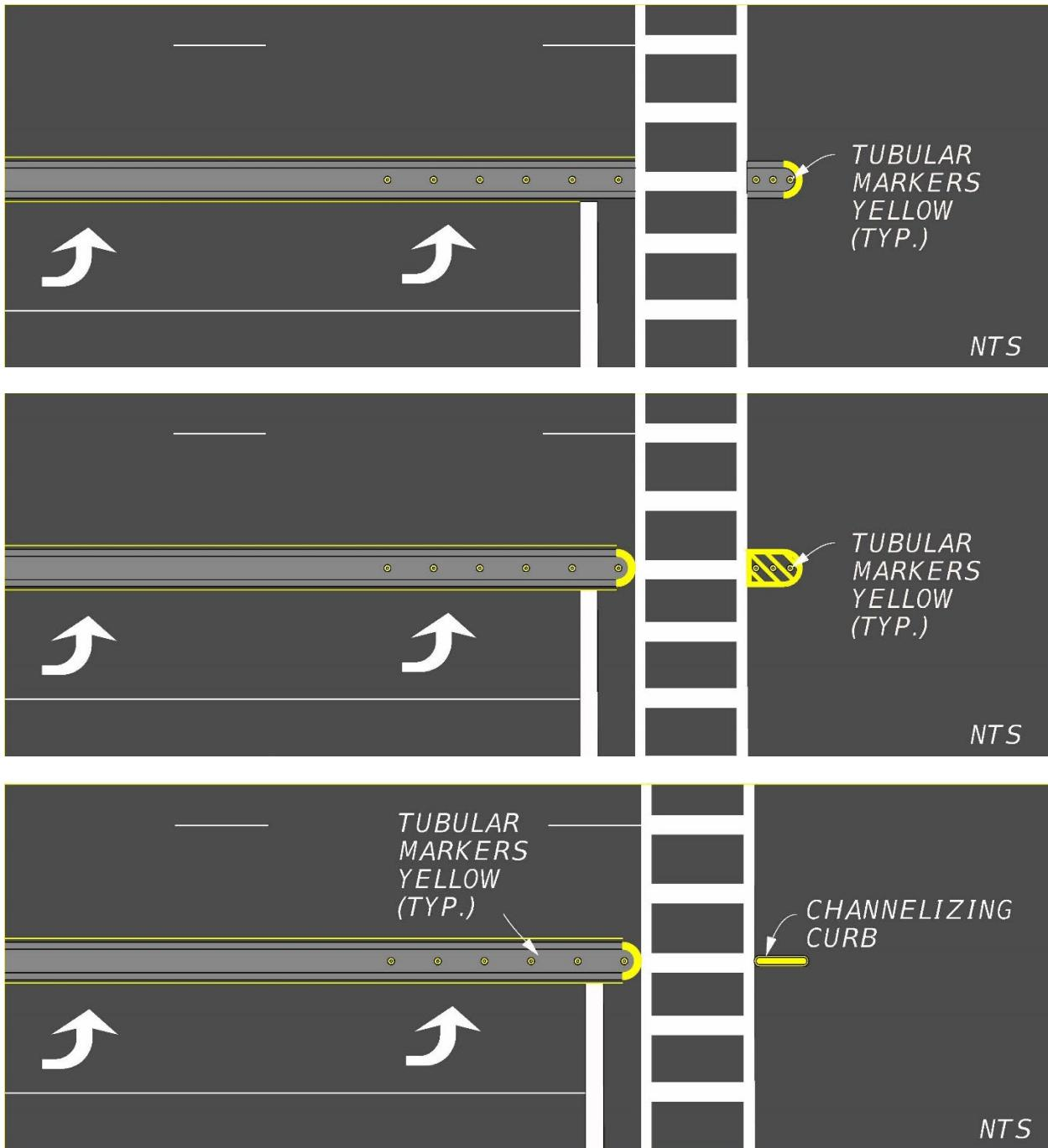
**Figure 210.3.7 Hardened Centerline without Traffic Separator**
