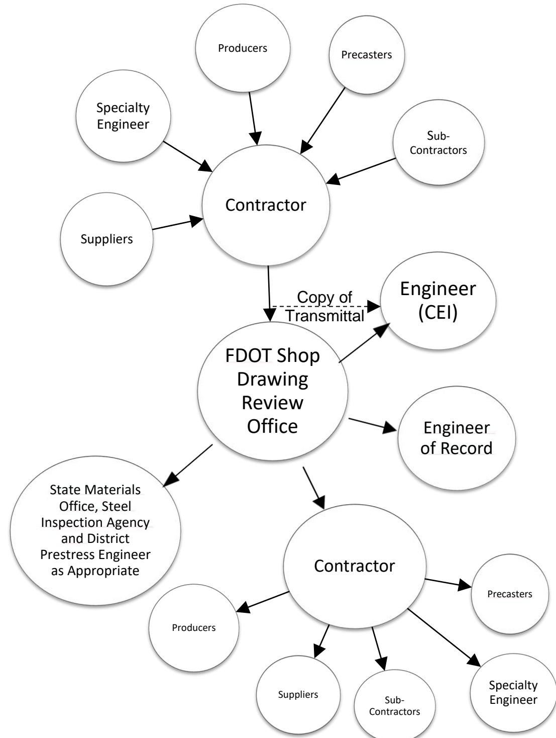
**Figure 152.11.4    Shop Drawing Flow Diagram for Design-Build Project- Shop Drawings Affecting Public Safety**
