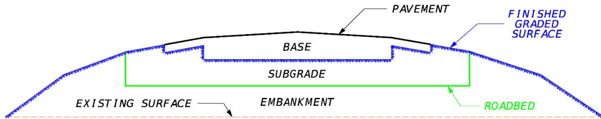
Projects are constructed over natural topography (Case I) or over existing roadbeds (Case II). Project may also have sections where both Case I and Case II apply.
