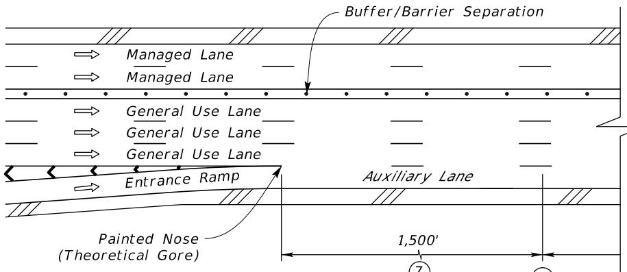
**Single-Lane Ramp with Auxiliary Lane Configuration**
