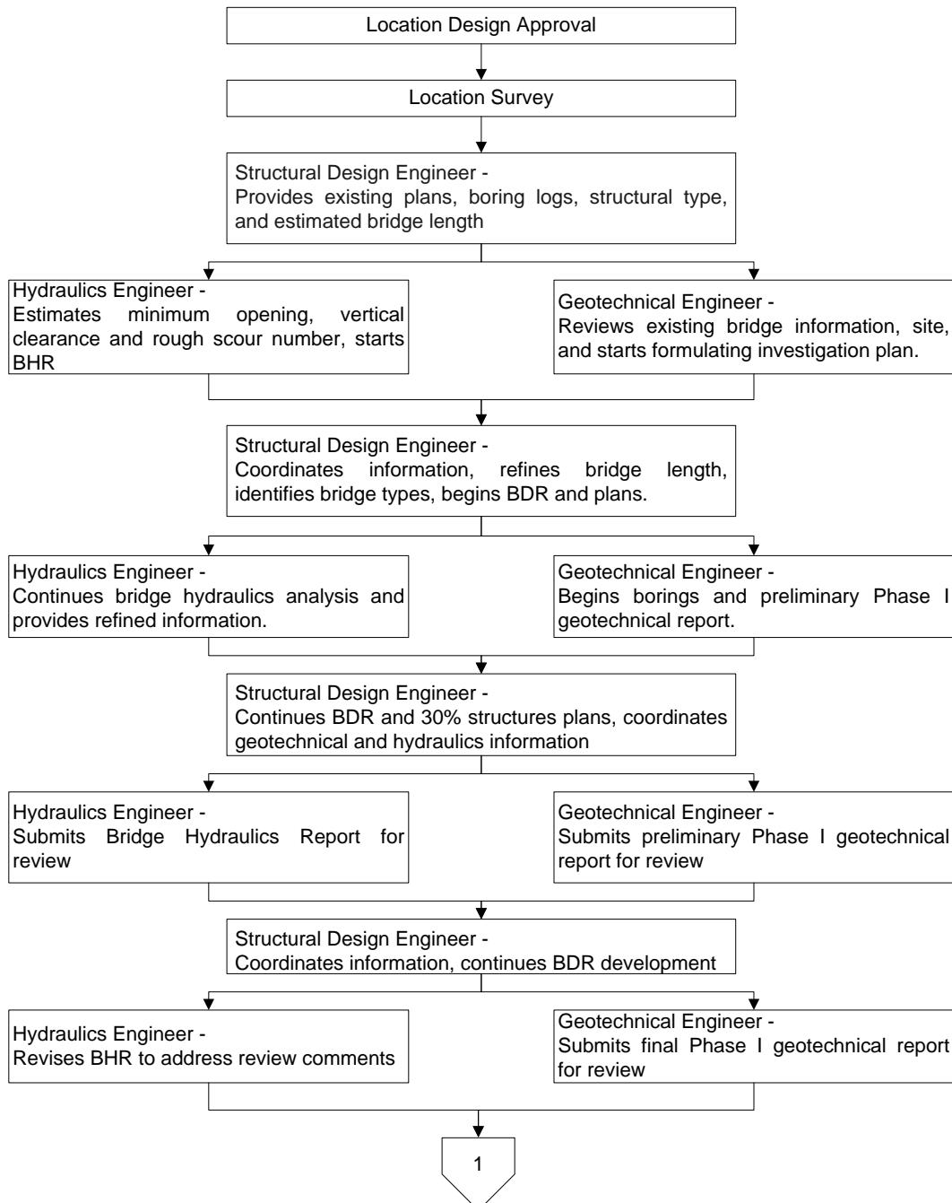
**Figure 250.2.1 Structural Plans Development**
