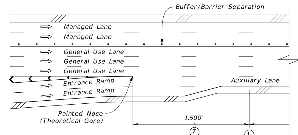
**Two-Lane Ramp with Auxiliary Lane Configuration**
