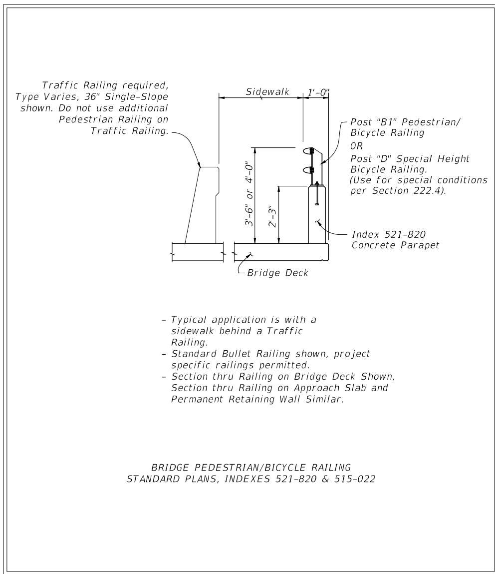
**Figure 222.4.3 Bridge Railing – Pedestrian/Bicycle Railing**
