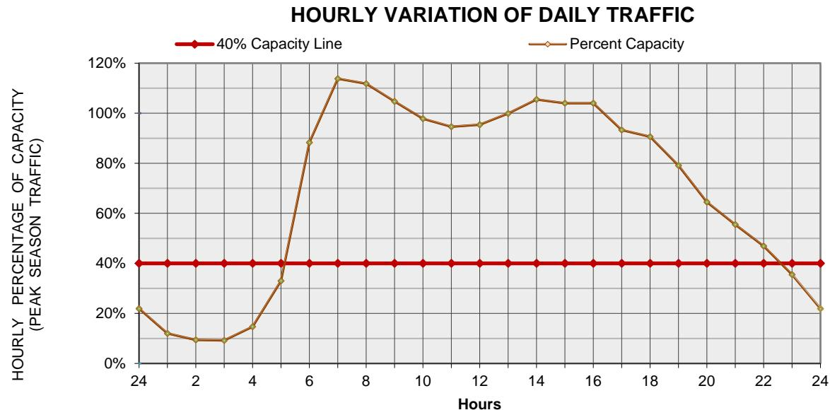
**STEP 2:** Identify the traffic pacing restrictions. Leave a buffer period of one hour between the end of traffic pacing operations and the beginning of 40% capacity.
