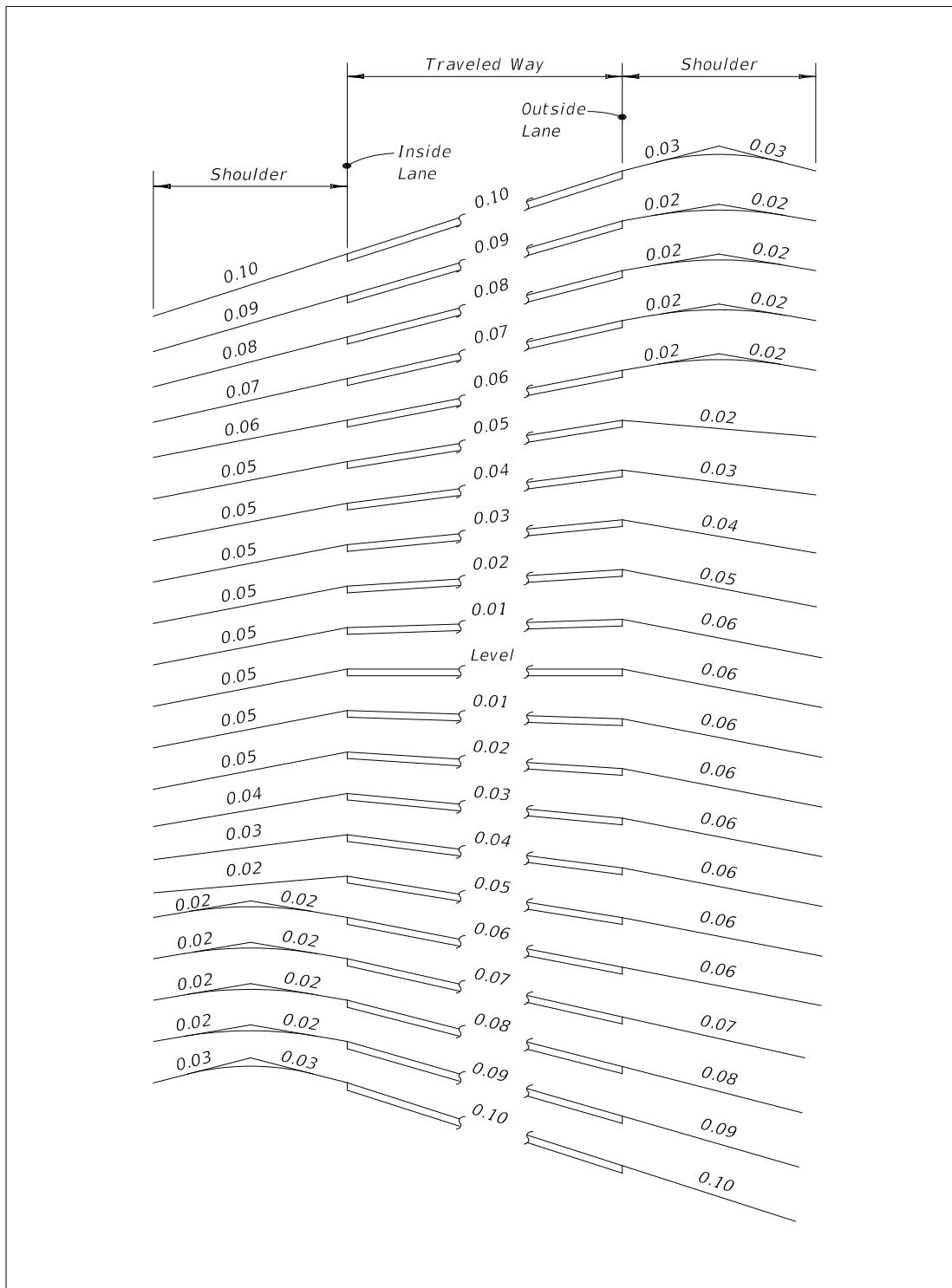
**Figure 211.4.2 Special Ramp Shoulder Superelevation**
