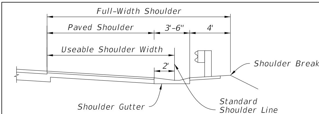
On resurfacing projects where paved or usable shoulder widths are less than 10 feet, do one of the following:
