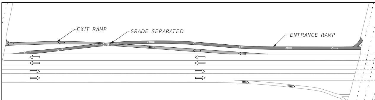
When combining general use lane or general toll lane exits and managed lane exits in a braided ramp configuration, the managed lane exit merges on the right side of the general use lanes or general toll lanes as illustrated in **Figure 211.12.3**. Operational analysis determines the actual lane configuration. Refer to **Traffic Analysis Handbook** and **Interchange Access Request User's Guide** for guidance on analysis requirements.
