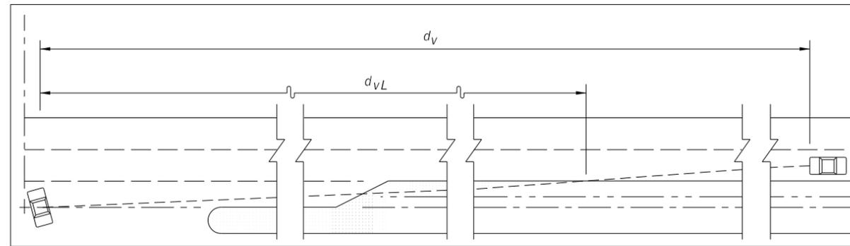
Where The Median Is Sufficiently Wide For The Design Vehicle To Pause In The Median (Vehicle Length Plus 6' Min.) The Clear Line Of Sight To The Right (d<sub>v</sub>) Is Measured From The Vehicle Pause Location, i.e., Not From The Cross Road Stop Position; Distances d<sub>r</sub> & d<sub>m</sub> Do Not Apply.
