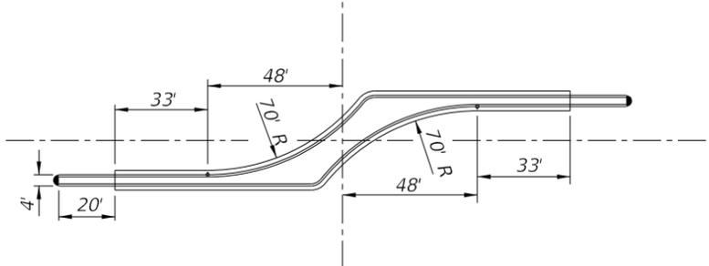
**NOTE:** Return configurations for each quadrant must be analyzed independently to assure adequate return pavement for semi-trailer inside tracking and for 4' minimum clearance between trucks making opposing movement. The depicted design only applies where roads and streets intersect at 90° to the mainline and have centerlines common with the opposing road or street. Swept paths are by AutoTURN 4.0 for the AASHTO 2001 WB-50 tractor-semitrailer.
