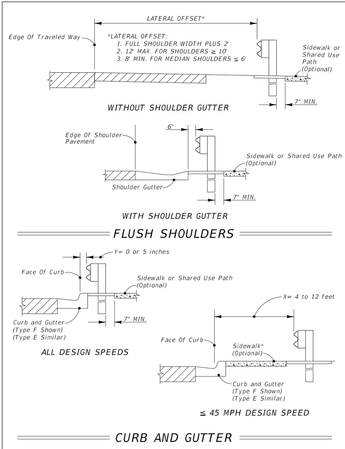
In addition to travel lane lateral offset considerations, an adequate setback must be provided behind the barrier to ensure proper function. Setback is the distance between the face of the barrier and the aboveground hazard behind the barrier. For flexible and semi-rigid barriers, the setback is based on deflection tolerances and is required to prevent the barrier from contacting aboveground hazards or breakaway devices.
