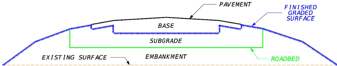
Projects are constructed over natural topography (Case I) or over existing roadbeds (Case II). Project may also have sections where both Case I and Case II apply.
