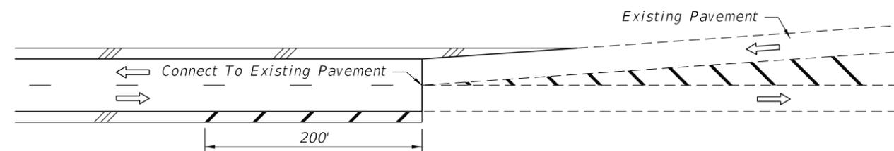
CONNECTING ROADWAY WITH PAVED SHOULDERS TO EXISTING ASYMMETRICAL FLARE WITHOUT PAVED SHOULDERS
