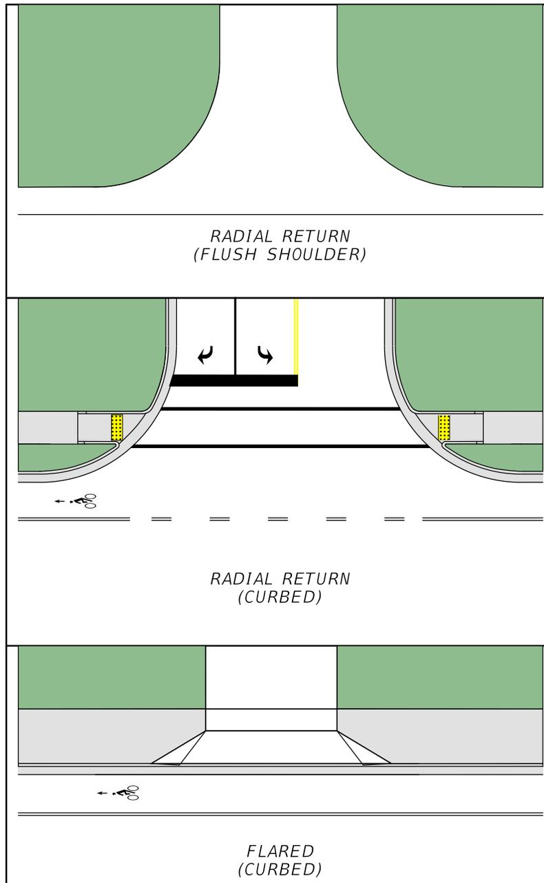
Determine the type of driveway needed based on roadway type (curbed or flush shoulder) and driveway traffic volumes. Flared driveways are used on curbed roadways where driveway traffic does not exceed 600 trips per day or 60 trips per hour (i.e., Connection Categories A and B) as shown in **Table 214.2.1**. Radial return designs are used on all flush shoulder roadways and on curbed roadways with driveway traffic greater than 600 trips per day (i.e., Connection Category C and D).
