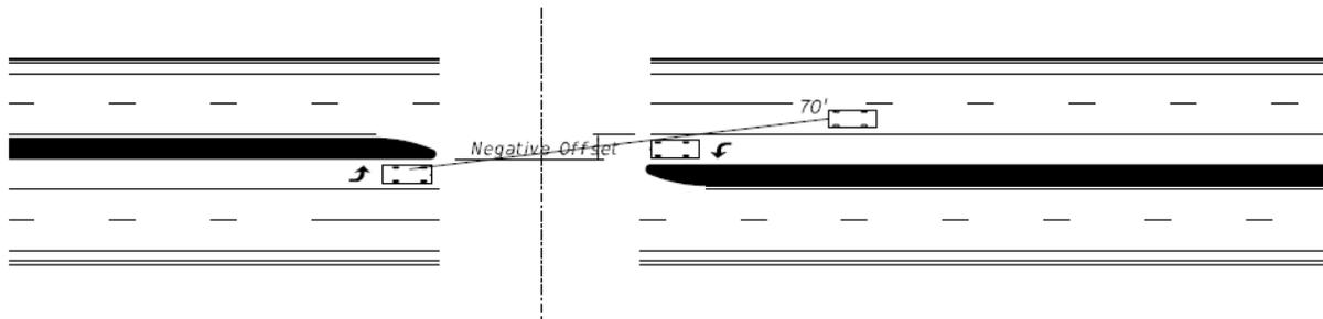
On curbed roadway designs, offset left-turn lanes should be used with median widths greater than 18 feet. A 4-foot traffic separator should be used when possible to channelize the left turn and provide separation from opposing traffic.
