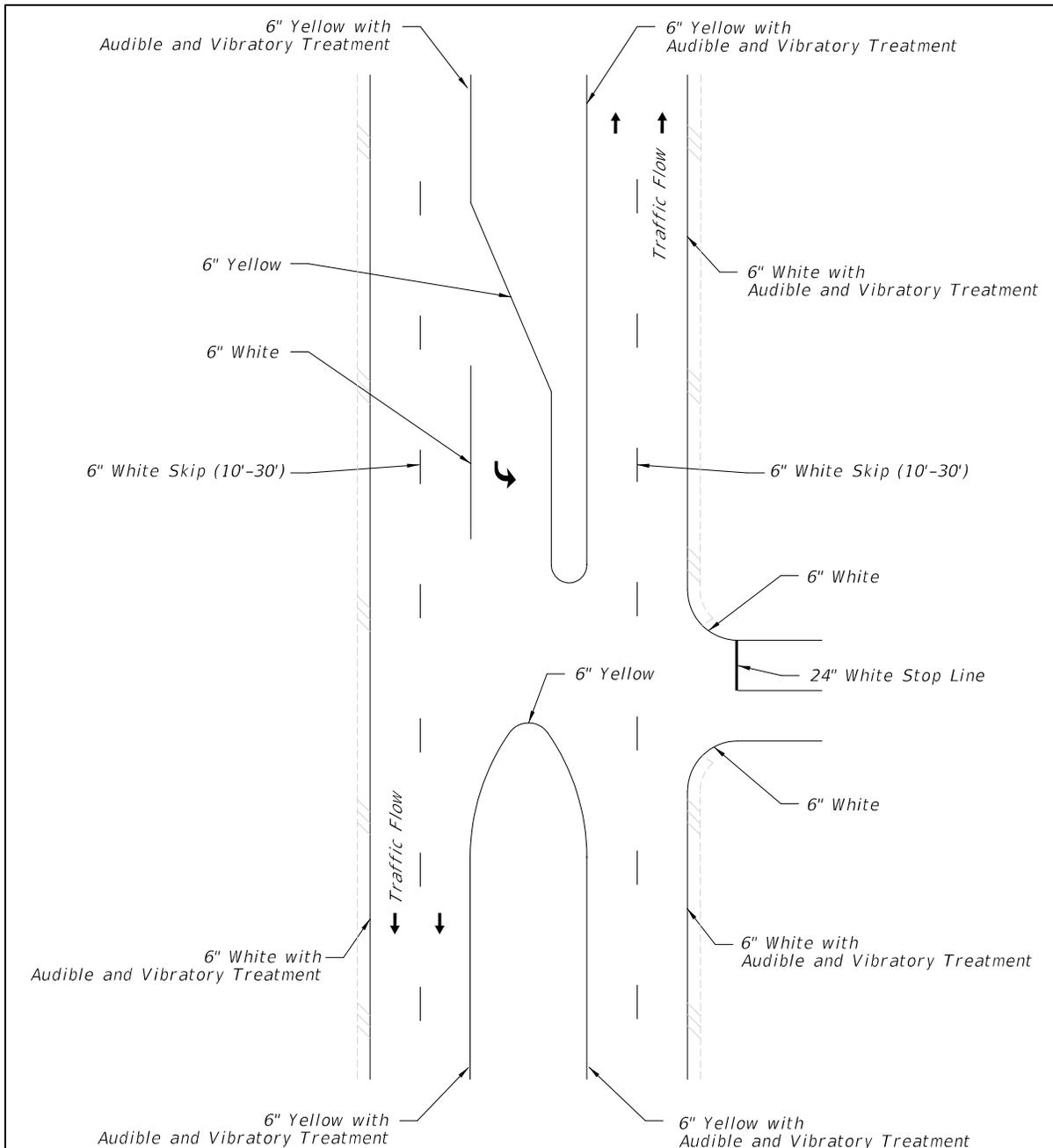
**Figure 210.4.4 Audible and Vibratory Treatment Placement (Cont.)**
