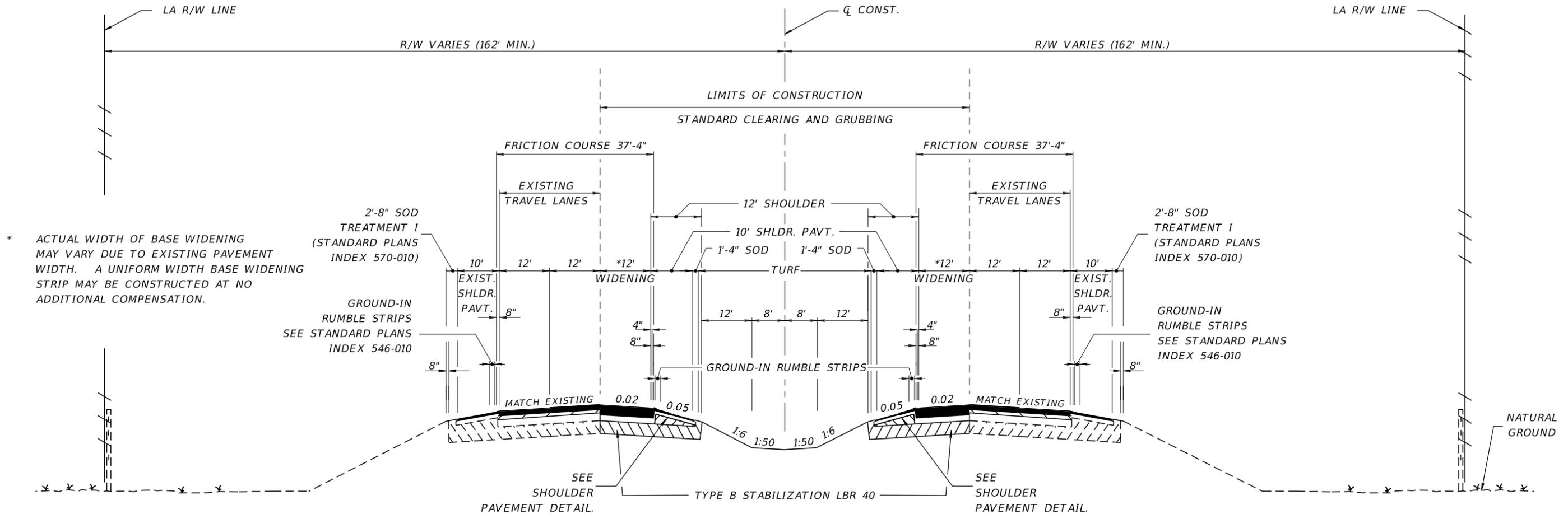
\* ACTUAL WIDTH OF BASE WIDENING MAY VARY DUE TO EXISTING PAVEMENT WIDTH. A UNIFORM WIDTH BASE WIDENING STRIP MAY BE CONSTRUCTED AT NO ADDITIONAL COMPENSATION.
