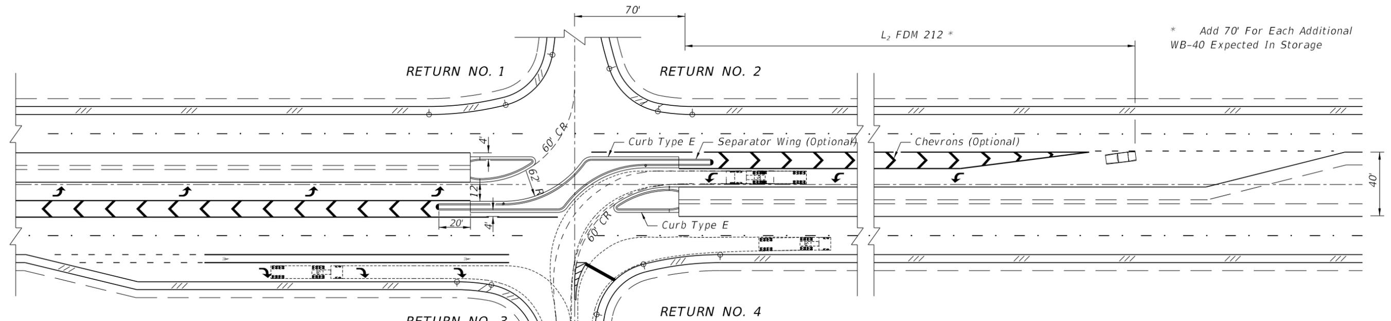
**NOTE:** Return configurations for each quadrant must be analyzed independently to assure adequate return pavement for semi-trailer inside tracking and for 4' minimum clearance between trucks making opposing movement. The depicted design only applies where roads and streets intersect at 90° to the mainline and have centerlines common with the opposing road or street. Swept paths are by AutoTURN 4.0 for the AASHTO 2001 SU and WB-40 tractor-semi-trailer.
