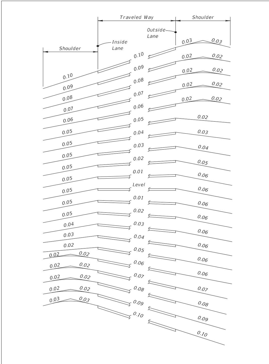
**Figure 211.4.2 Special Ramp Shoulder Superelevation**
