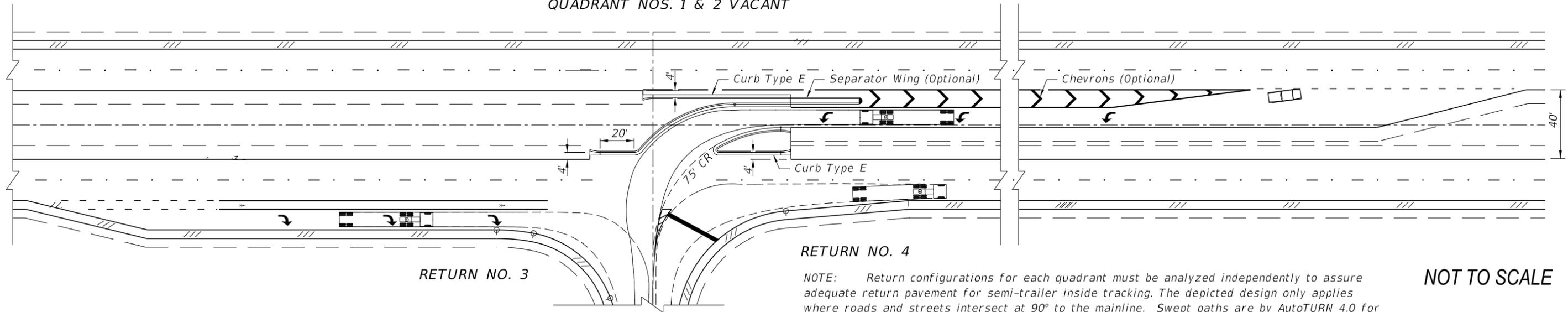
**NOTE:** Return configurations for each quadrant must be analyzed independently to assure adequate return pavement for semi-trailer inside tracking. The depicted design only applies where roads and streets intersect at 90° to the mainline. Swept paths are by AutoTURN 4.0 for the AASHTO 2001 WB-50 tractor-semitrailer.
