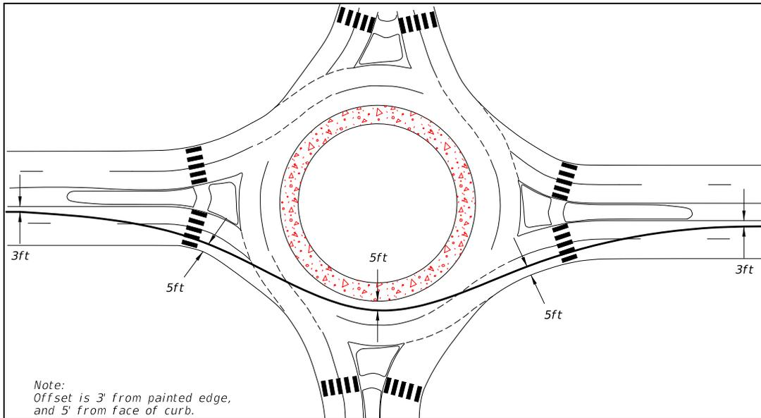
**Figure 213.6.2 Fastest Path for Right Turn Movement**
