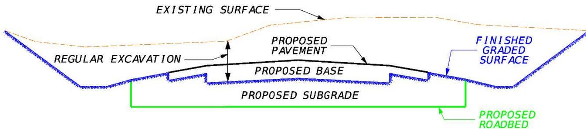
Calculate the Embankment quantities from the existing surface to the finished graded surface.
