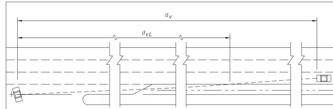
Where The Median Is Sufficiently Wide For The Design Vehicle To Pause In The Median (Vehicle Length Plus 6' Min.) The Clear Line Of Sight To The Right ( $d_v$ ) Is Measured From The Vehicle Pause Location, i.e., Not From The Cross Road Stop Position; Distances  $d_r$  &  $d_m$  Do Not Apply.
