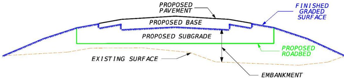
Case II projects may or may not include the removal of existing base material or removal of existing concrete pavement. According to [Standard Specification 120-4.2](#):
