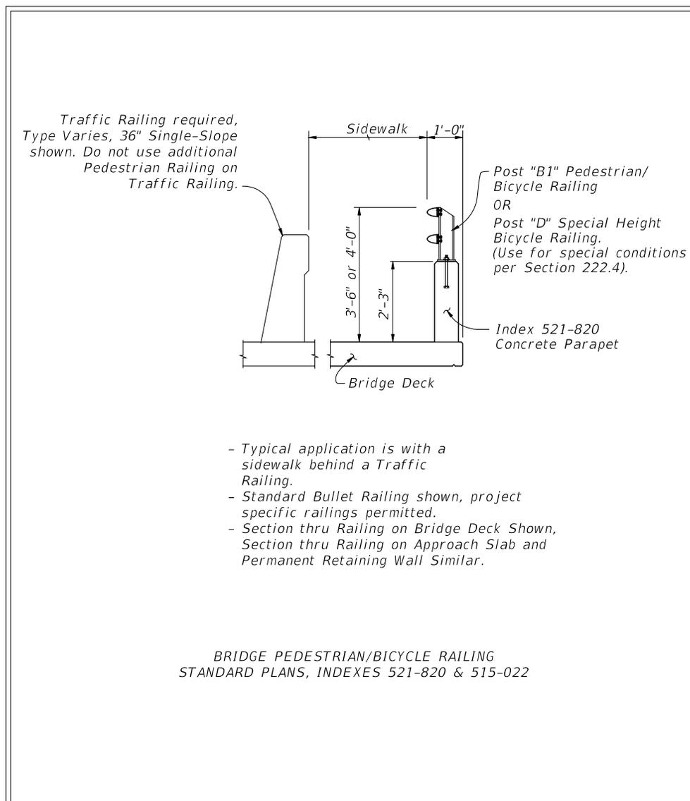
**Figure 222.4.3 Bridge Railing – Pedestrian/Bicycle Railing**
