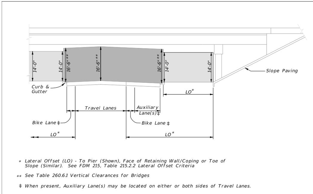
**Figure 260.6.4 Curbed Roadway  $\leq 45$  mph – Section through Bridge**
