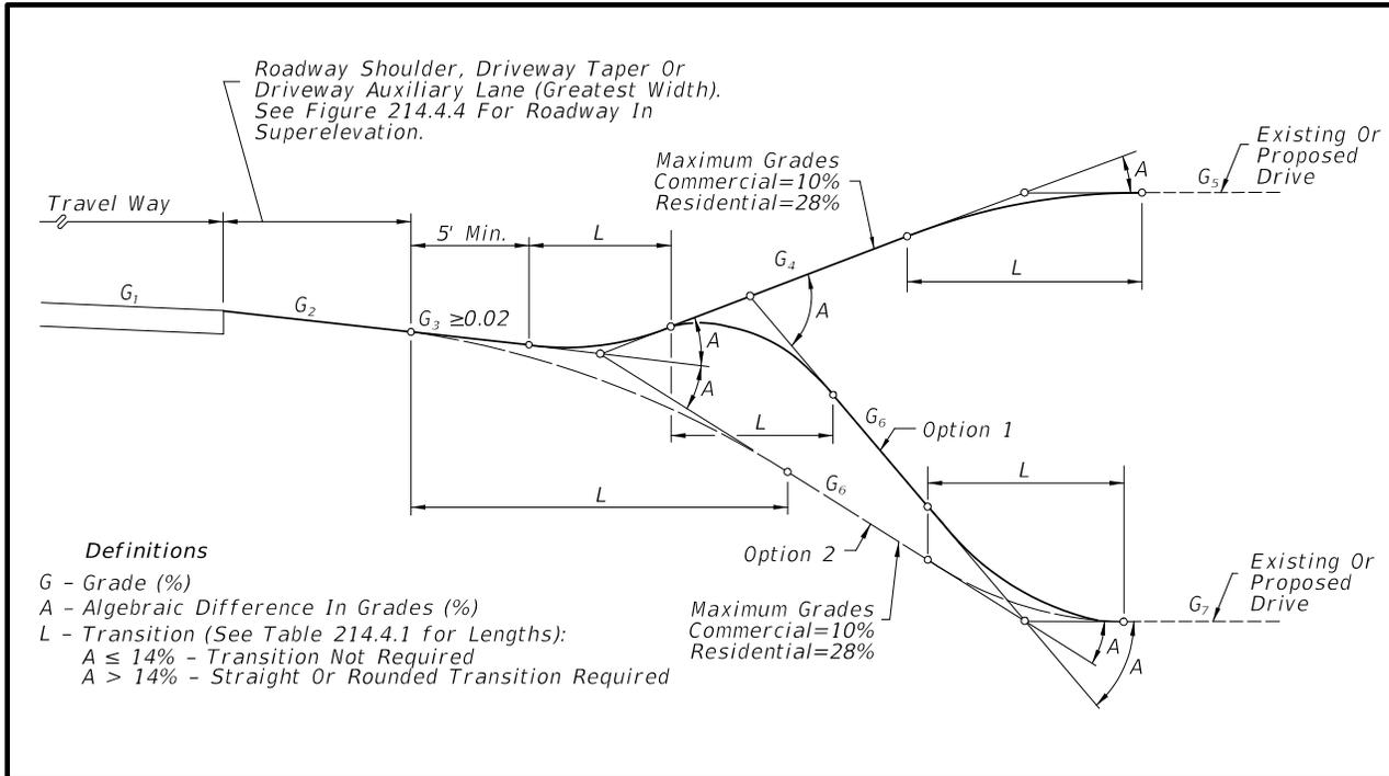
**Figure 214.4.4 Driveway Slope for Flush Shoulder Roadway in Superelevation**
