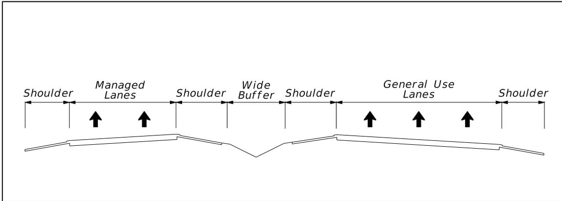
**Figure 211.3.4 Managed Lanes Grade Separation Typical Section**
