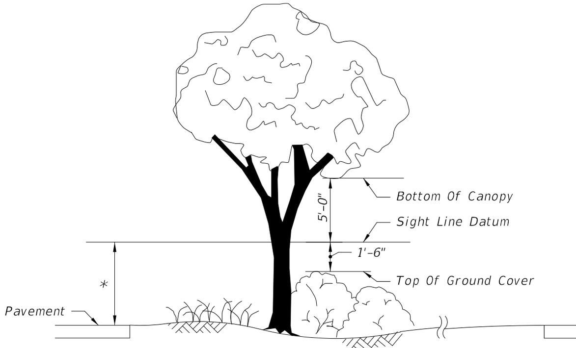
\* Since observations are made in both directions, the line of sight datum between roadways is 3.5 feet above both pavements.
