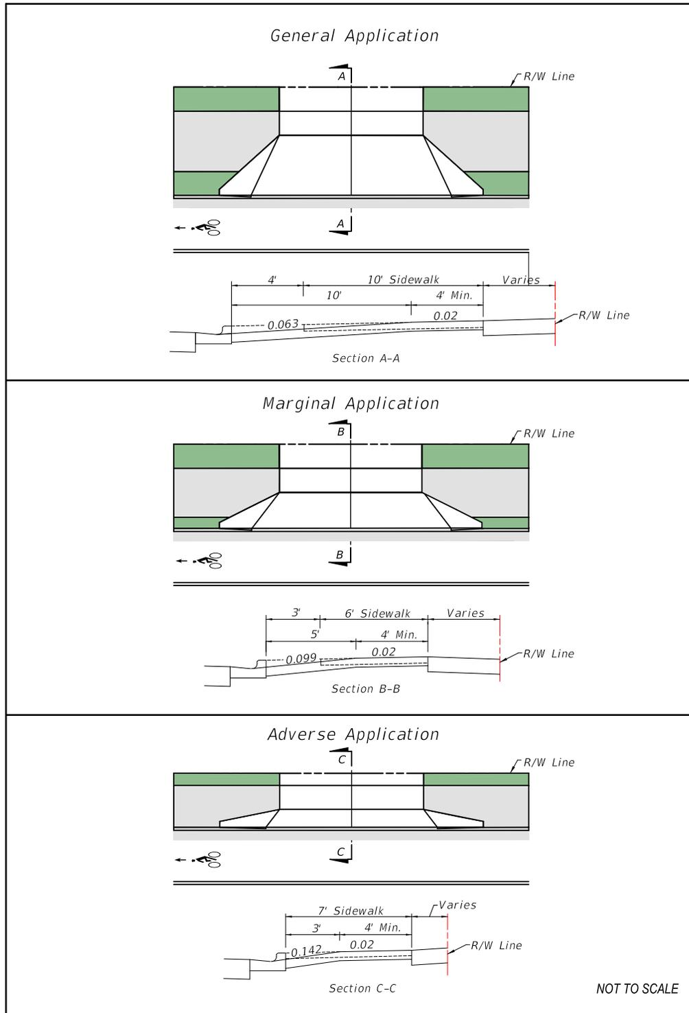
**Figure 214.4.2 Curbed Roadway Driveway Profiles**
