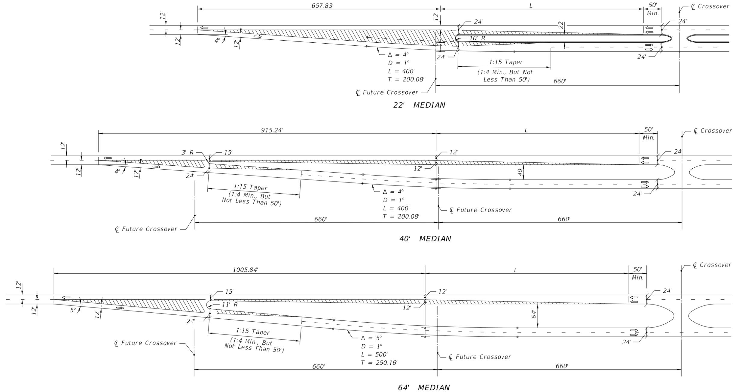
$$L = \frac{WS^2}{60} \text{ FOR DESIGN SPEEDS } \leq 40 \text{ mph}$$
