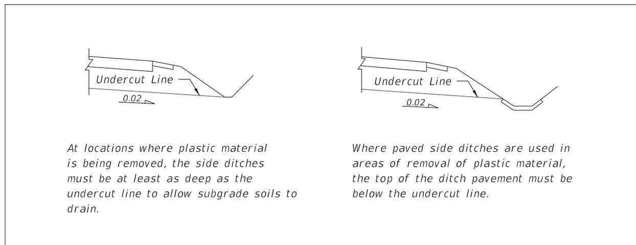
**Figure 216.4.8 Excavation and Embankment**
