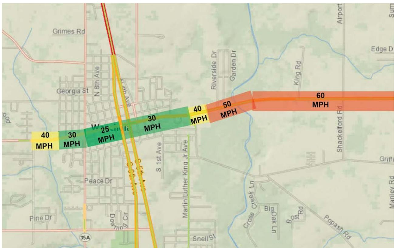
**Figure 202.4.4 Section Change Near Transition from 40 to 30 mph
