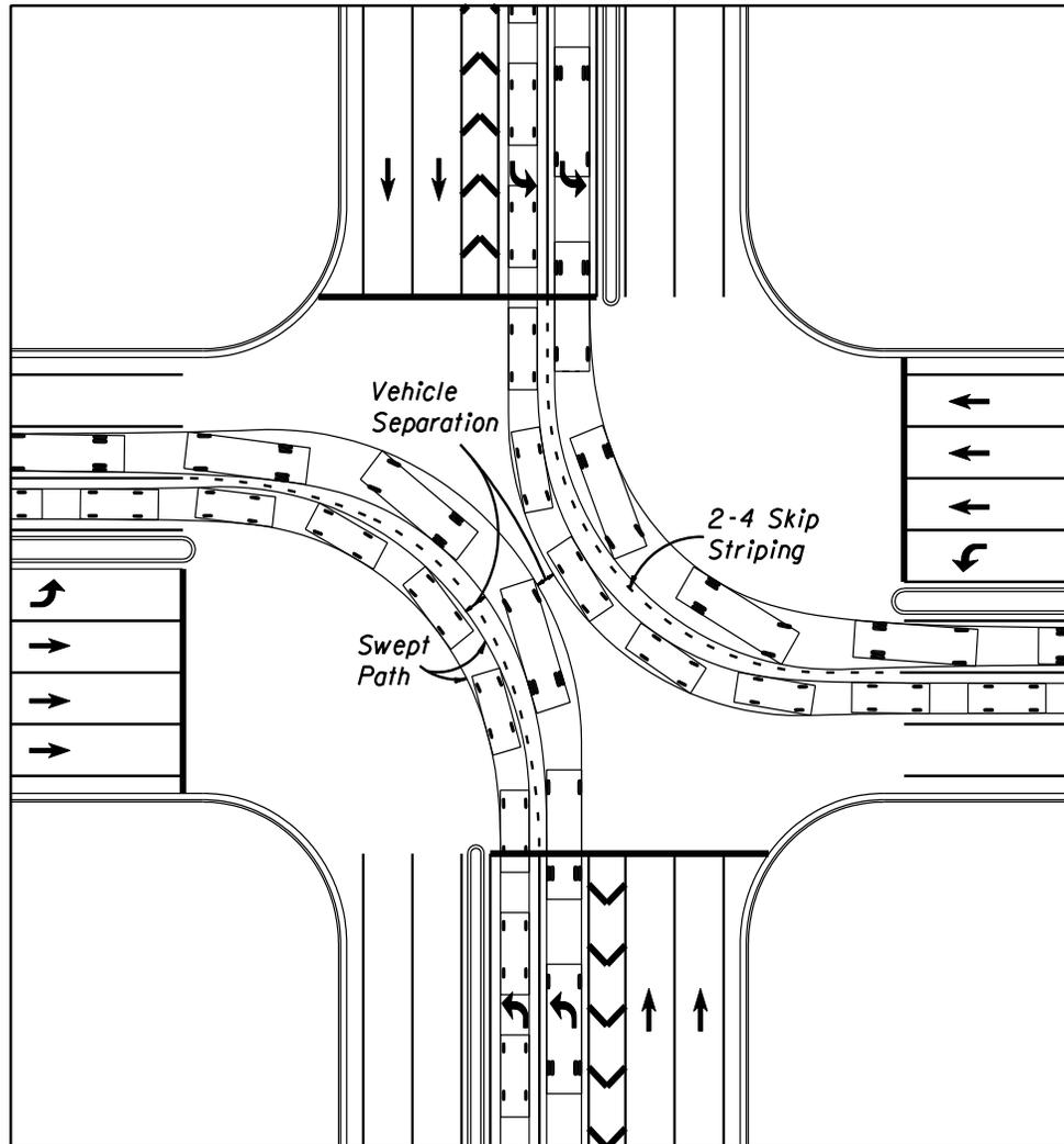
Design of triple left turns should accommodate a WB-62FL (outside lane), a SU-40 (center or inside lane), and a P vehicle (center or inside lane) turning simultaneously.
