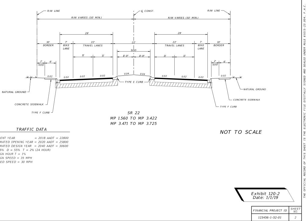
CURRENT YEAR ESTIMATED OPENING YEAR = 2020 AADT = 25800 ESTIMATED DESIGN YEAR = 2040 AADT = 30600 K = 6% D = 55% T = 2% (24 HOUR) DESIGN HOUR T = 1%DESIGN SPEED = 35 MPH POSTED SPEED = 30 MPH
