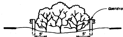
CROSS SECTION BACK TO BACK GUARDRAIL
