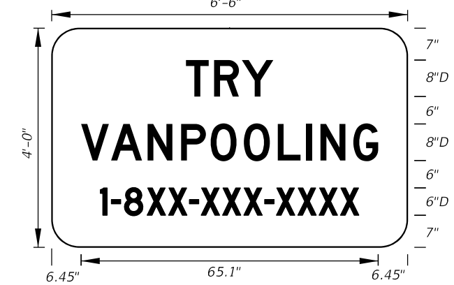
FTP-57-06 6'-6" X 4' 6" Radii 8" and 6" Series D Legend Blue Background White Legend and Border Design Project Manager or Transit Administrator will supply correct 1-8XX number.
