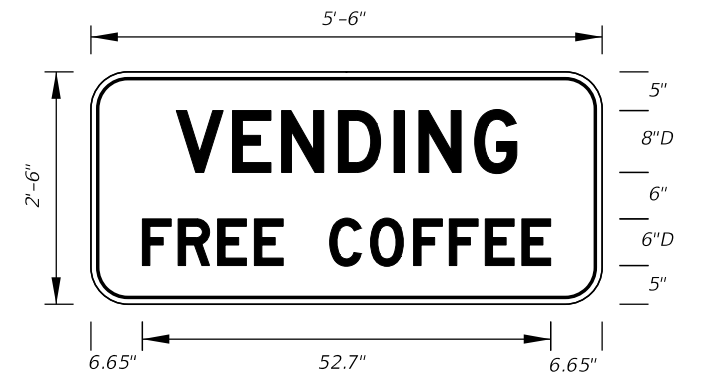
FTP-74-06 5'-6" X 2'-6" 4" Radii 3/4" Border 6" Series D Legend Blue Background White Legend and Border
