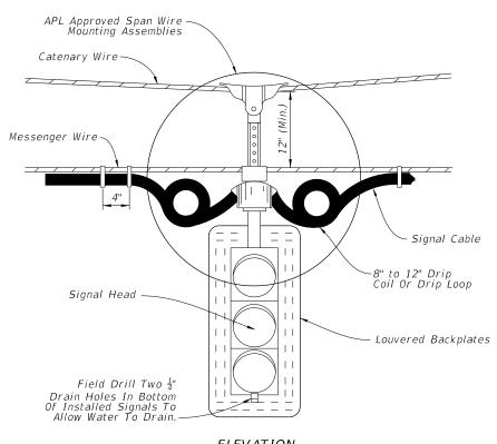
ELEVATION SIGNAL ATTACHMENT
