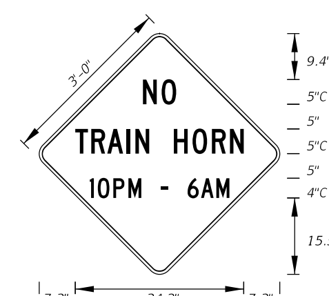
FTP-62-06 3' X 3' 2" Radii 3/4" Border 4" and 5" Series C Legend Yellow Background Black Legend and Border
