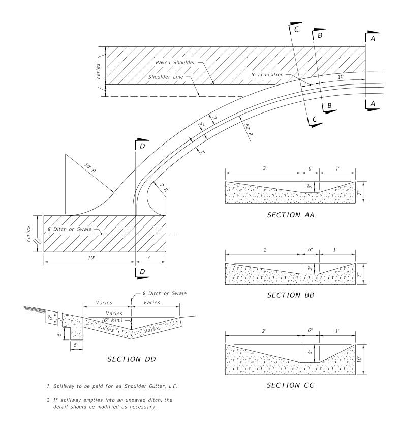
DETAIL OF CONCRETE SPILLWAY AT END OF SHOULDER GUTTER (TO BE USED WHERE INLETS, PIPES & ENDWALLS ARE IMPRACTICAL)
