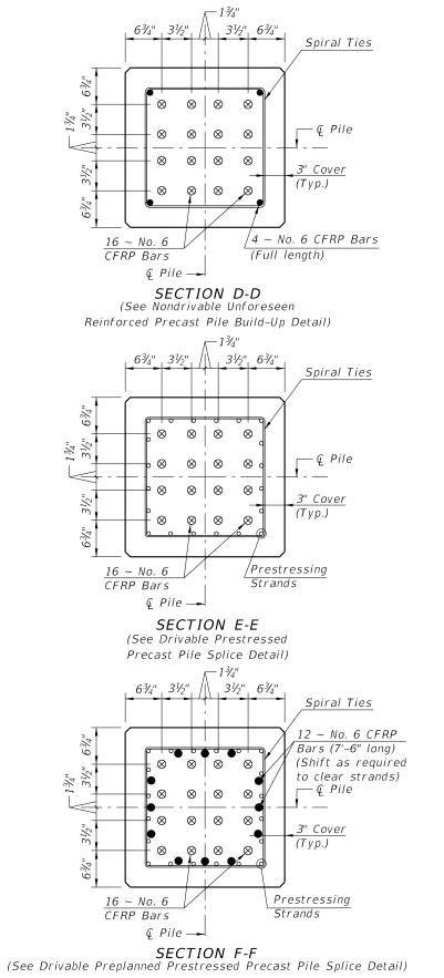
CFRP PILE SPLICE REINFORCEMENT DETAILS
