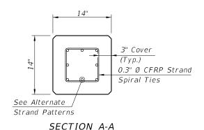
Spiral Ties @ 6" pitch, full length 13/4" 3" Cover (Typ.)4 ~ No. 6 4 ~ No. 6 CFRP Bars CFRP Bars (Full Length) Ç Pile →
