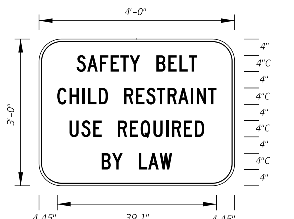
FTP-45-06 4' X 3' 5" Radii 3/4" Border 4" Series C Legend White Background Black Legend and Border
