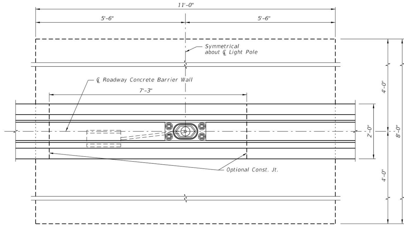
Provide dowel bars @ construction joint
