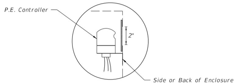
Cut a 2" hole in the side of the Lighting Control Panel enclosure for the operation and mounting of the P.E. controller. Use plexiglass and a clear silicone sealant to cover hole, install P.E. Controller.
