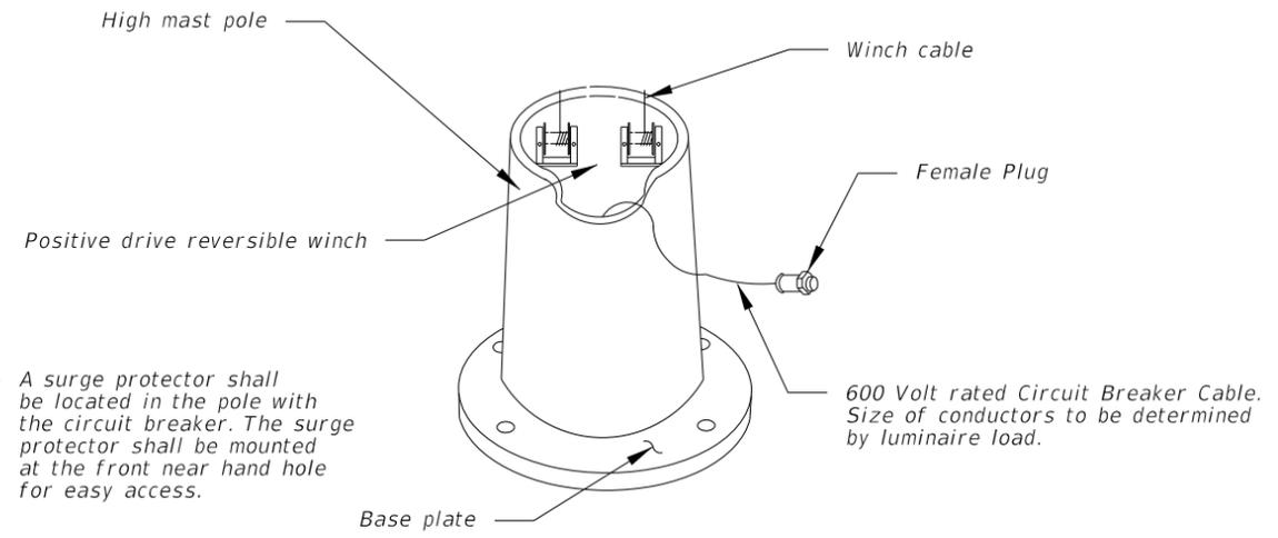
A surge protector shall be located in the pole with the circuit breaker. The surge protector shall be mounted at the front near hand hole for easy access.
