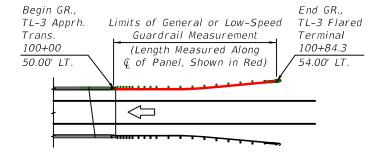
GUARDRAIL LENGTH MEASUREMENT EXAMPLE:
