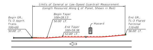
GUARDRAIL LENGTH MEASUREMENT EXAMPLE:
