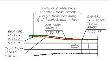
GUARDRAIL LENGTH MEASUREMENT EXAMPLE:
