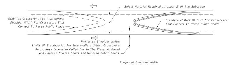
Limits Of Stabilization For Intermediate U-turn Crossovers And, Unless Otherwise Called For In The Plans, At Paved And Unpaved Private Roads And Unpaved Public Roads. Stabilize Crossover Area Plus Normal Stabilize Crossover Area Plus Normal Shoulder Width For Crossovers That Shoulder Width For Crossovers That Connect To Paved Public Roads Connect To Paved Public Roads
