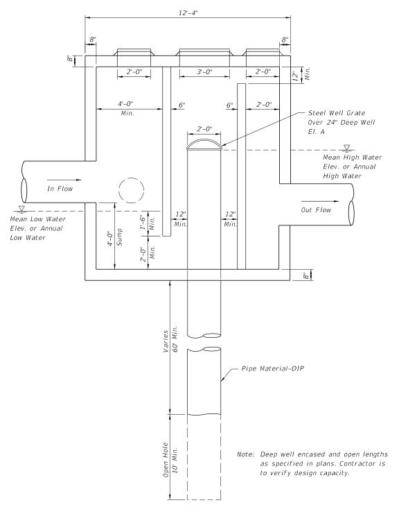
SPECIAL MANHOLE STRUCTURE DETAIL WITH OUTFALL
