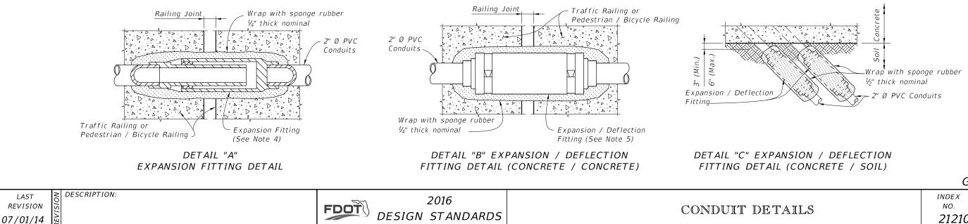
\* Reduce to 6" maximum when installed in Pedestrian/ Bicycle Railings.
