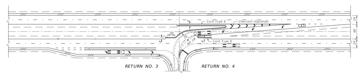
NOTE: Return configurations for each quadrant must be analyzed independently to assure adequate return pavement for semi-trailer inside tracking. The depicted design only applies where roads and streets intersect at 90° to the mainline. Swept paths are by AutoTURN 4.0 for the AASHTO 2001 SU and WB-40 tractor-semitrailer.
